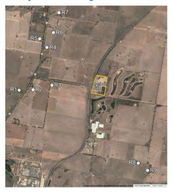
Attended noise measurements were undertaken at the site boundary to determine the existing ROBE facility operational noise emissions. The measurements were undertaken:
