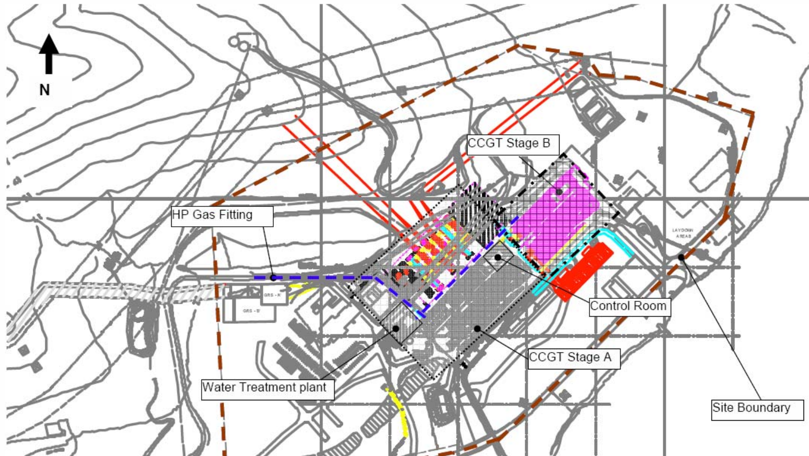
■ Figure 3-3 Site layout of typical combined cycle gas turbine power station
