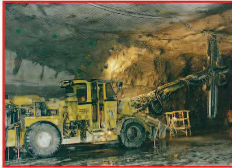
Installing rock bolts to provide roof support
