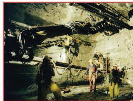
Loading explosives into drill holes
