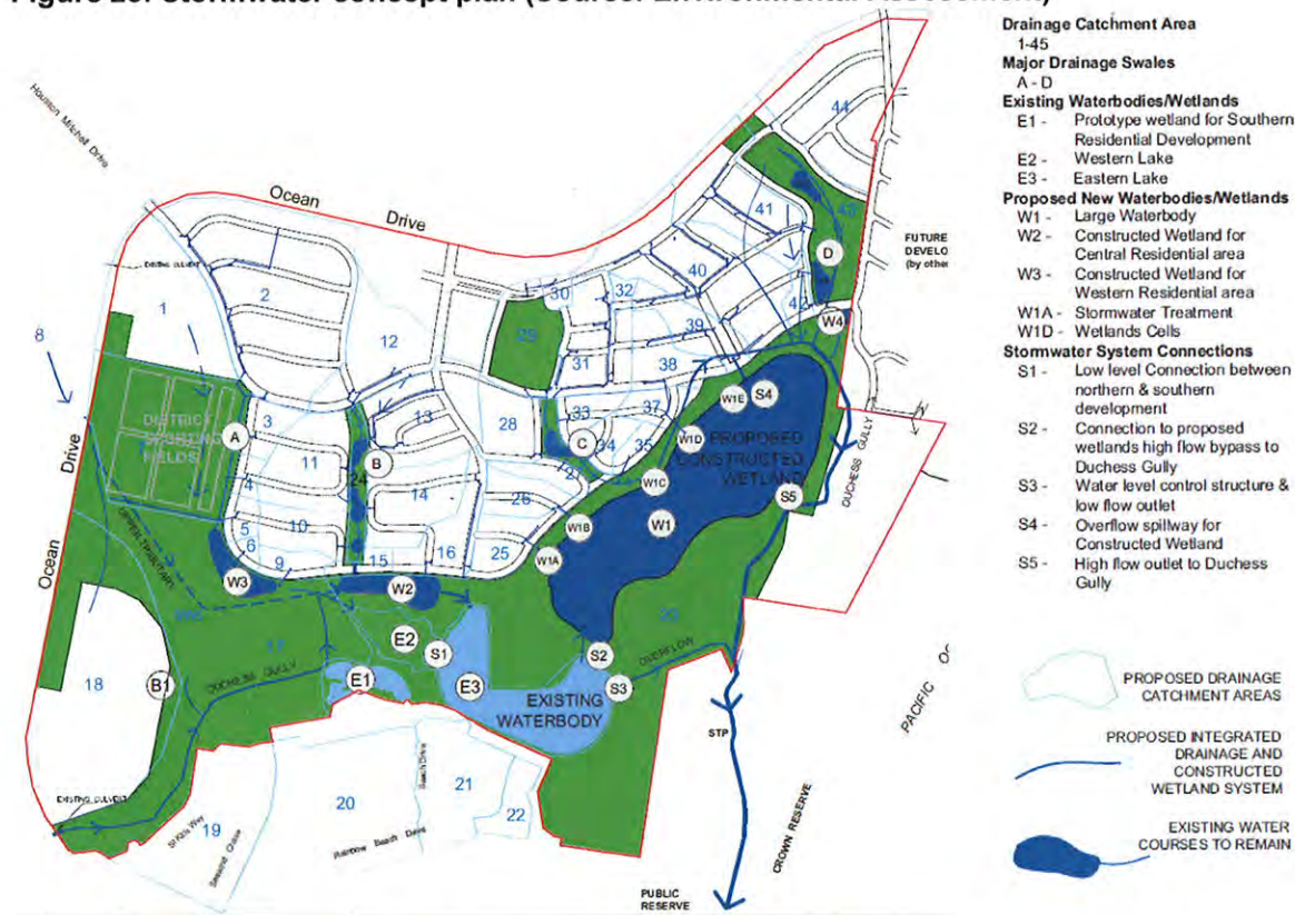
Figure 23: Stormwater concept plan (Source: Environmental Assessment)
