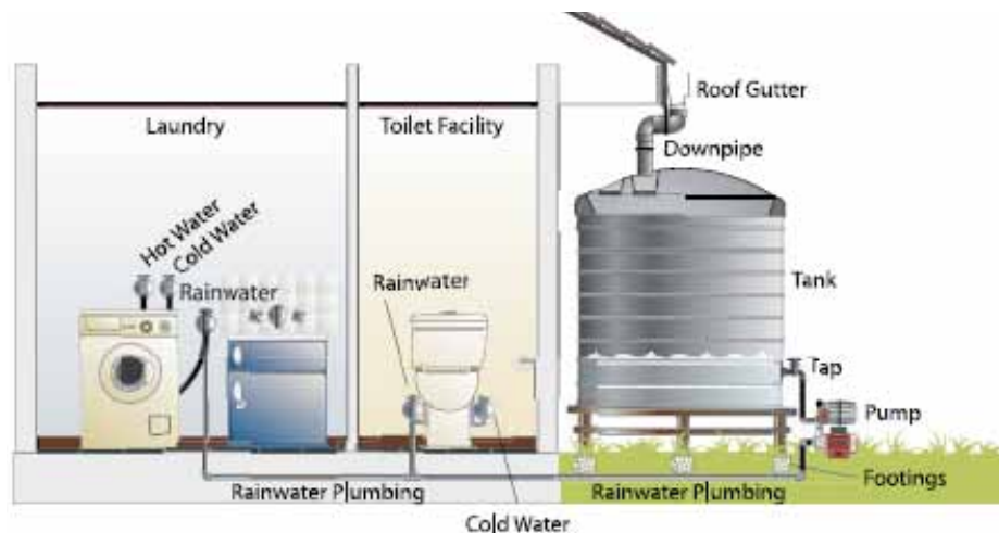
Figure 1: Typical configuration of a rainwater tank used to meet / supplement laundry and toilet water demands (ACT Government, 2006)
