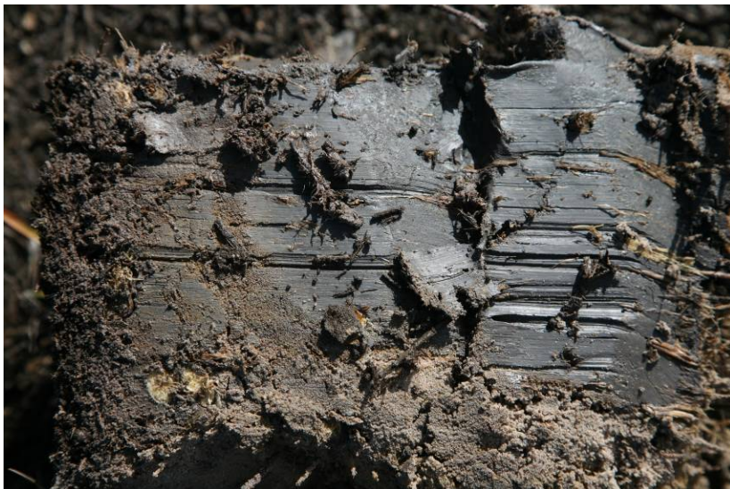
Figure 7 Heavy plastic clay dug from the surface of the Marshland. The low permeability of this soil is thought to be responsible for the impeded drainage of the Marshland.
