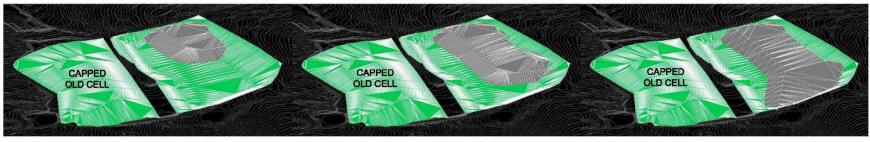
CAPACITY = 131, 634m<sup>a</sup> CELL 1 LIFE = 4.38 YEARS COST = CAPACITY = 124, 781m<sup>3</sup> CELL 2 LIFE = 4.16 YEARS COST = CAPACITY = 119, 121m<sup>3</sup> CELL 3 LIFE = 3.97 YEARS COST =
