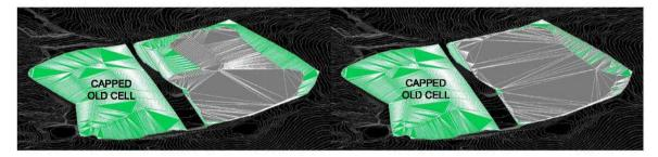
CAPACITY = 142, 096m<sup>3</sup> CELL 4 LIFE = 4.73 YEARS COST = CAPACITY = 142, 497m<sup>3</sup> CELL 5 LIFE = 4.74 YEARS COST =
