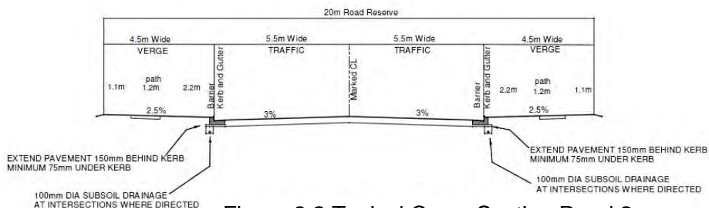
Figure 3.2 Typical Cross Section Road 2
