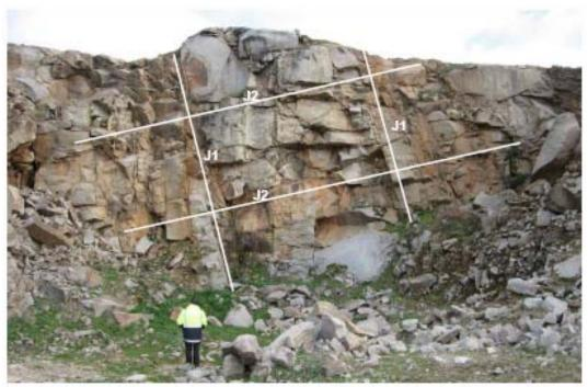
**Plate BM1:** Locality 1, Looking west at quarry face exposed at Blyth Merino Quarry showing the slightly weathered and fresh nature of the rock mass at this locality. The dominant joint sets are highlighted.
