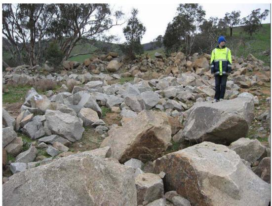
Plate BM3: Locality 2, Photo looking south-east at both fresh and slightly weathered granodiorite blocks, note equidimensional, oblique-shaped nature of the rock blocks. These rocks were sampled and crushed for material testing.
