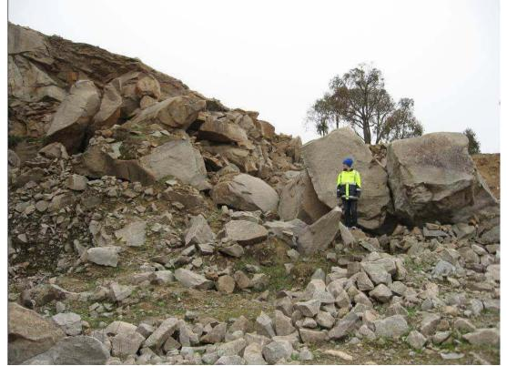
**Plate BM2**: Locality 1, Photo looking north at variation in block size and oblique-shaped (rhomboidal) equidimensional rock blocks.
