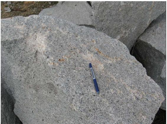
**Plate BM5:** Locality 2, Close up detail of ex-situ block of fresh granodiorite showing pale grey, evengrained and isotropic nature of the rock mass. The white and pale grey minerals are plagioclase feldspar and quartz and the black flecks are biotite.
