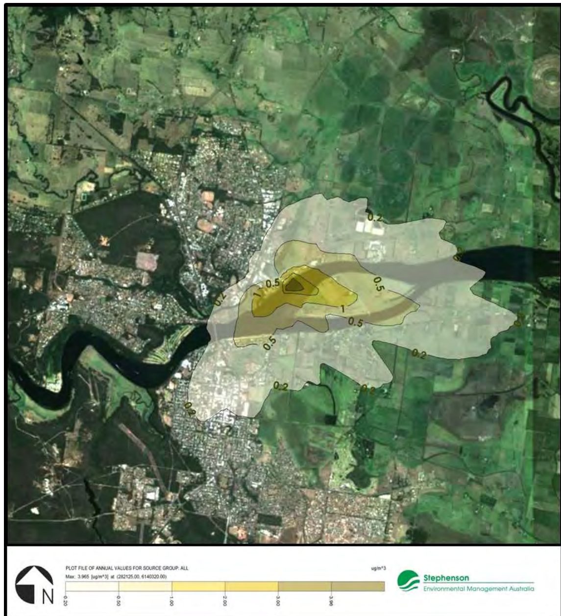
FIGURE 6-2 PREDICTED TSP CONCENTRATION RELOCATED DRYER, SHOALHAVEN STARCHES
