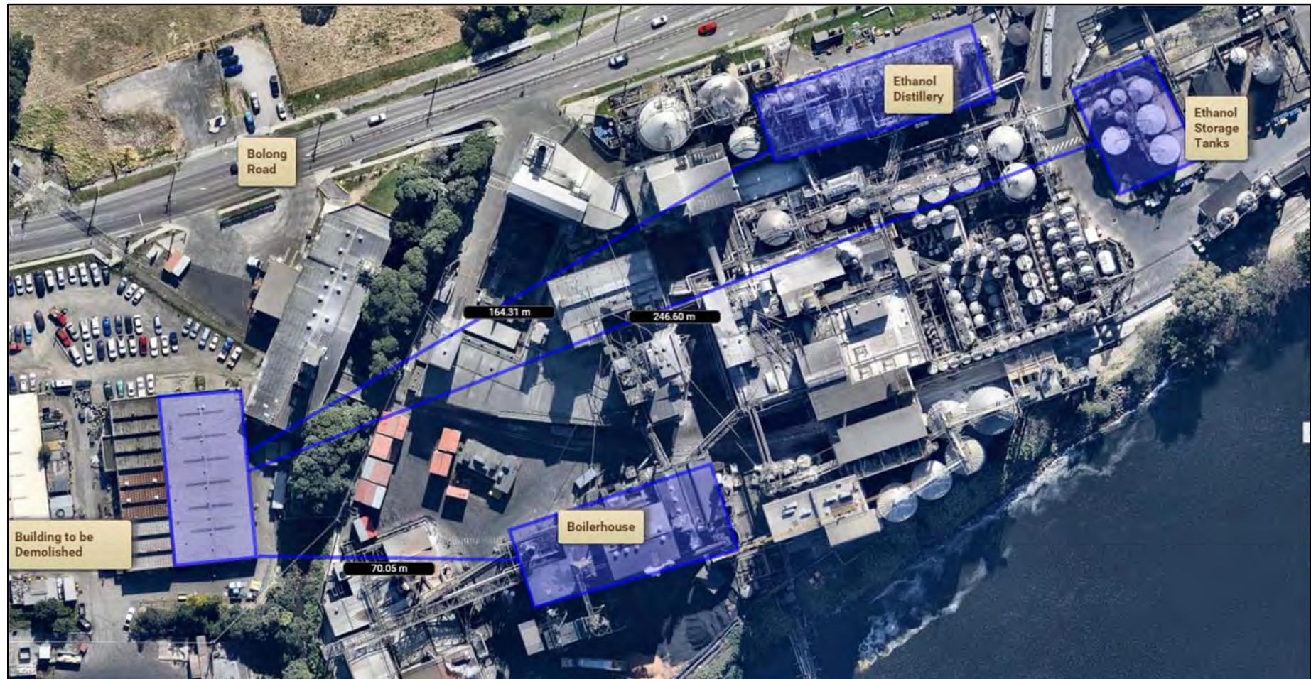
Figure 13: Proximity of building to be demolished in relation to hazardous locations within Shoalhaven Starches factory site.
