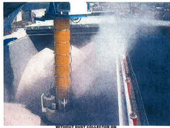
Figure 3 - A load chute with dust extractor switched off
