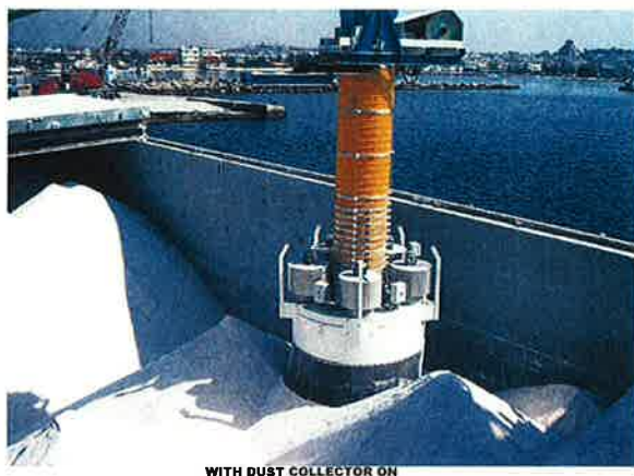
Figure 2 - A load-chute with dust extractor operating
