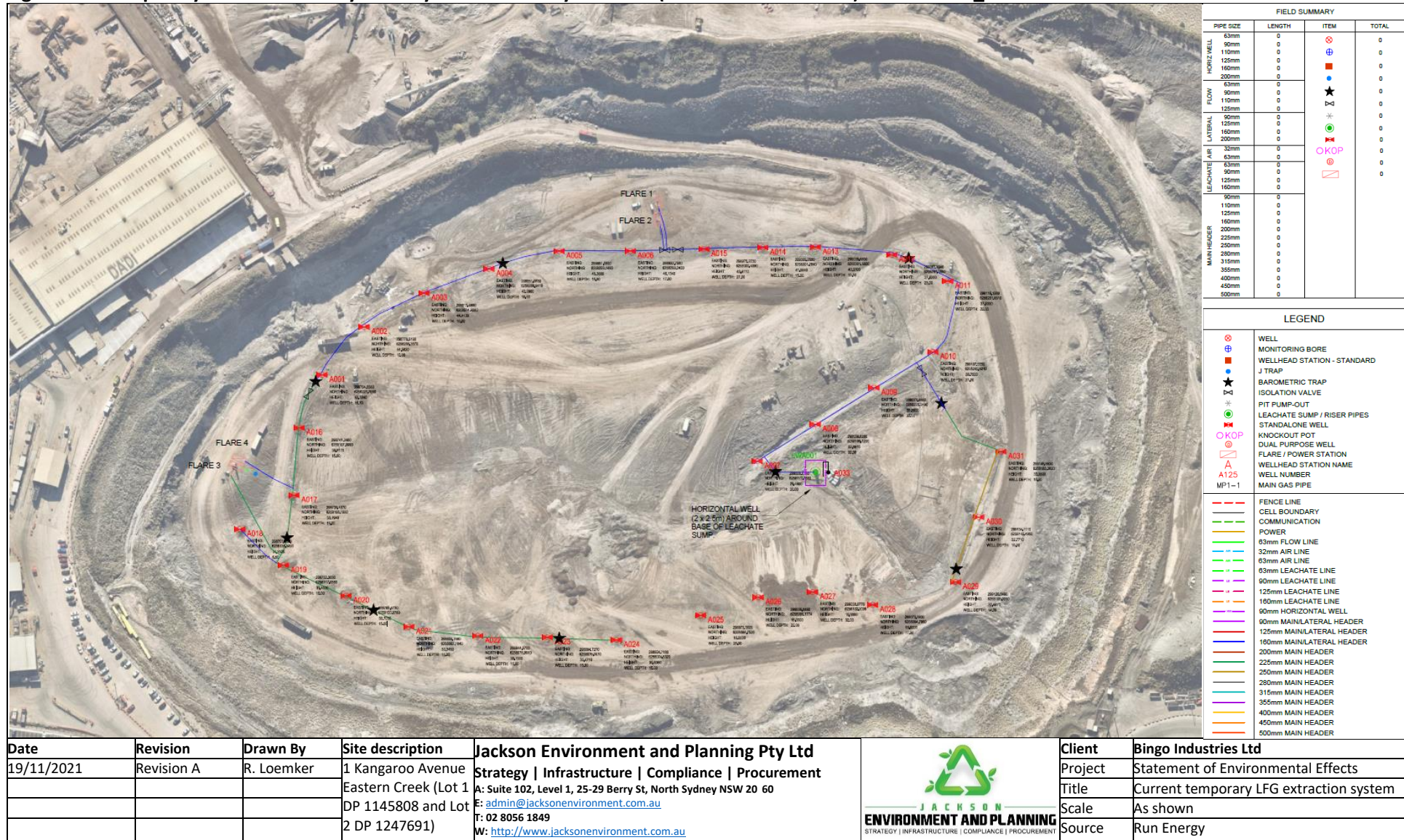
Figure 2.4. Temporary LFG extraction system layout as currently installed (as of November 2021) under MP06_139.
