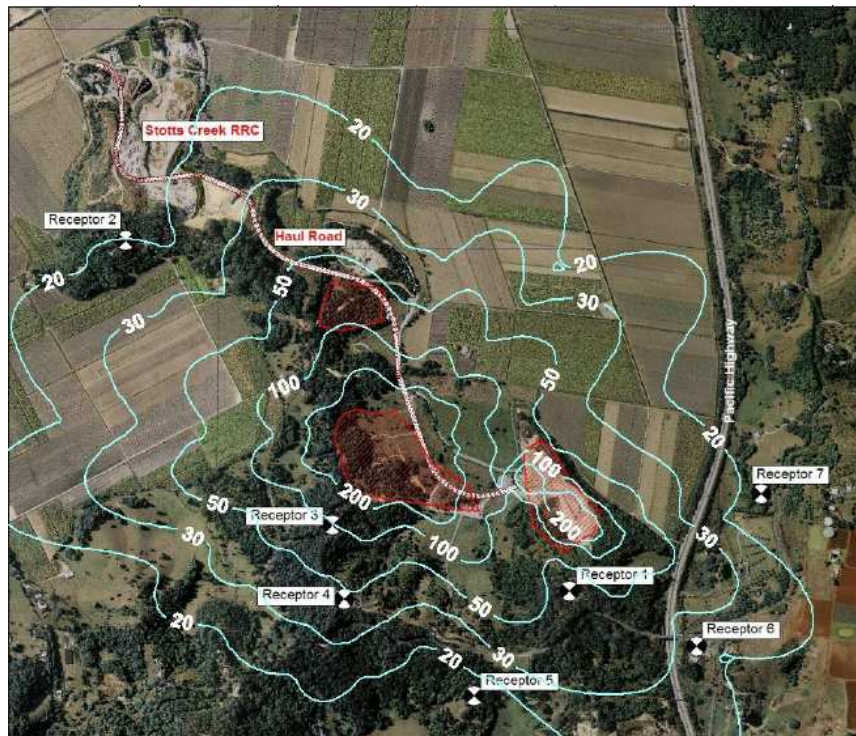
Figure 8: Configuration 1 (Stage 1) – PM 10 24-hour concentration contours
