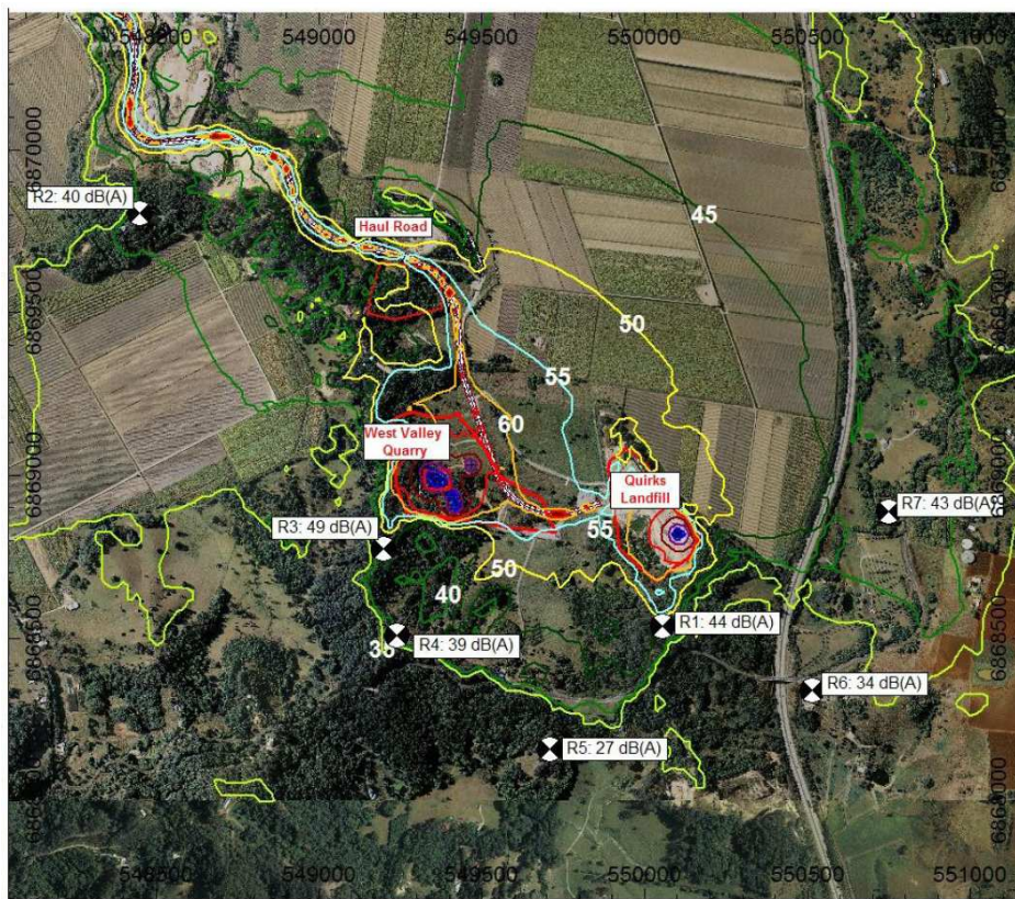
Figure 9: Configuration 1 (Stage 1) – Noise Contours
