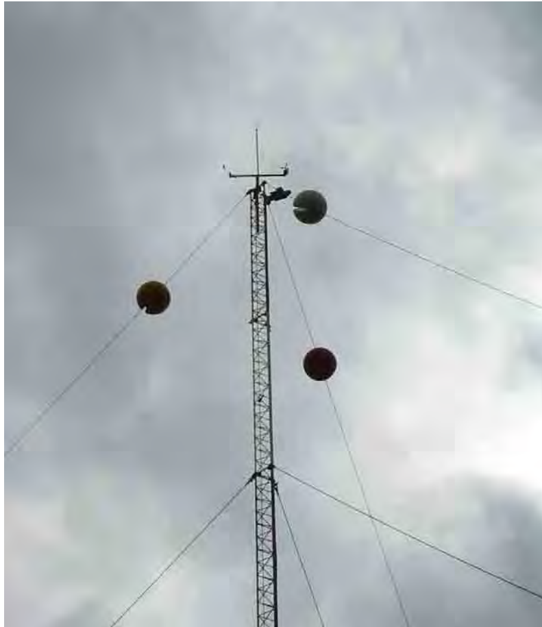
Figure 2.3 - Mounting of the anemometer and wind and wind vane installed at a height of 45m agl. A Data logger is installed closer to the base of the tower for logging ten minute mean wind speed and direction, standard deviation and maximum wind speeds.
