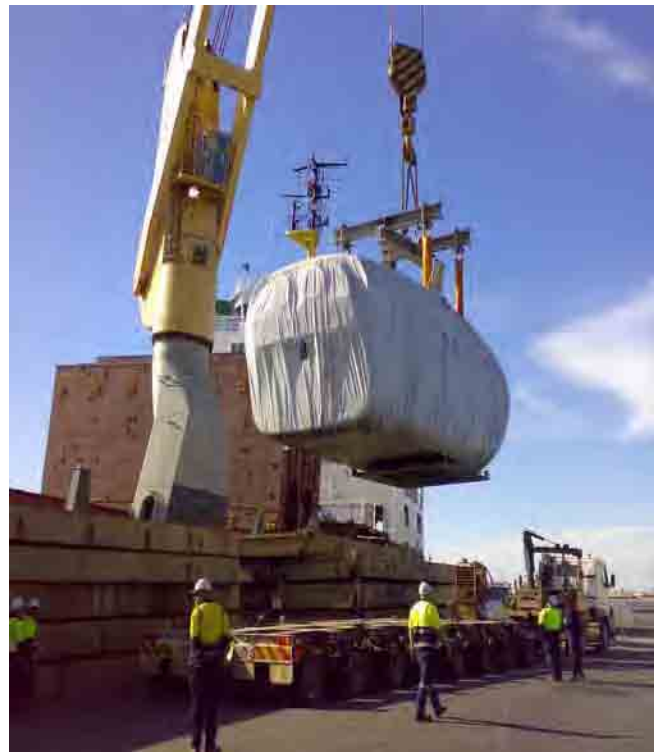
Unloading a Wind Turbine Generator at Port
