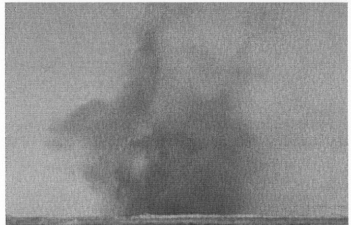
Figure 1 – Oxides of nitrogen generated by blasting
