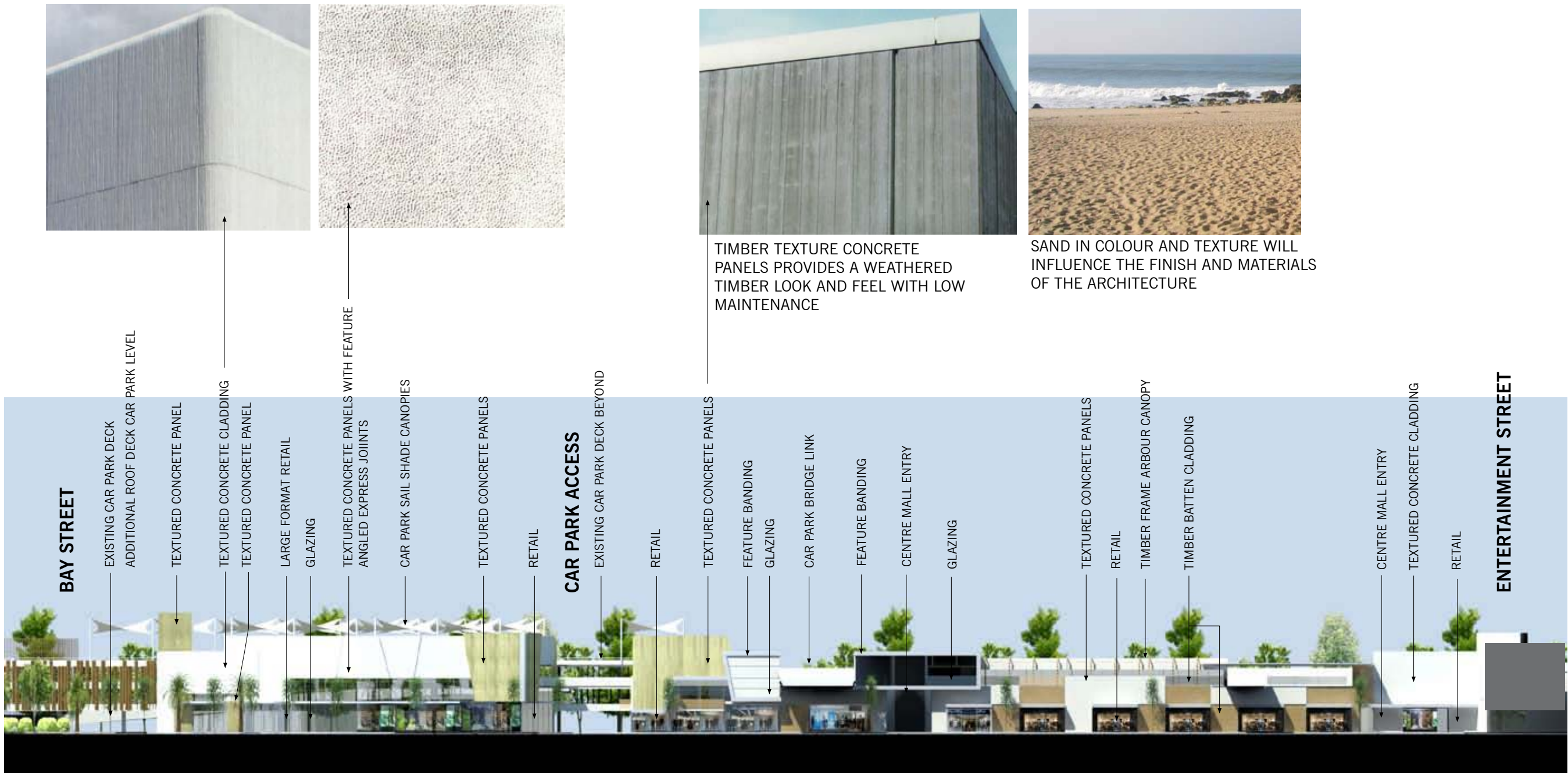
LEISURE STREET ELEVATION - WEST
