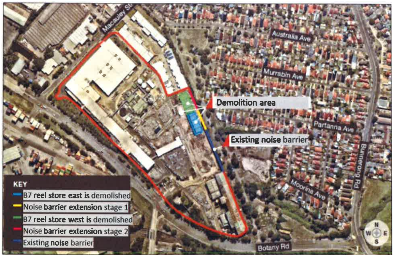
Figure 4 | Proposed staged demolition and noise barrier extension
