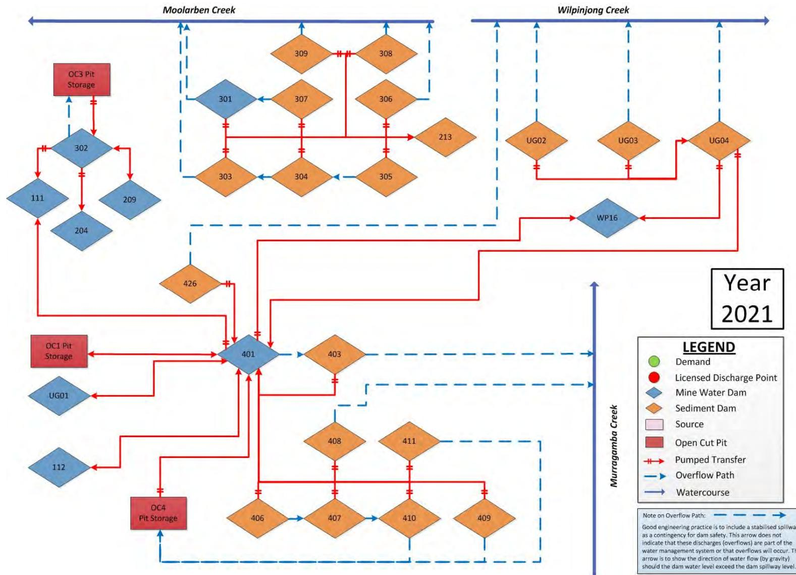
Figure 5.5 - Water management system schematic - OC3 and OC4 (Phase 2)
