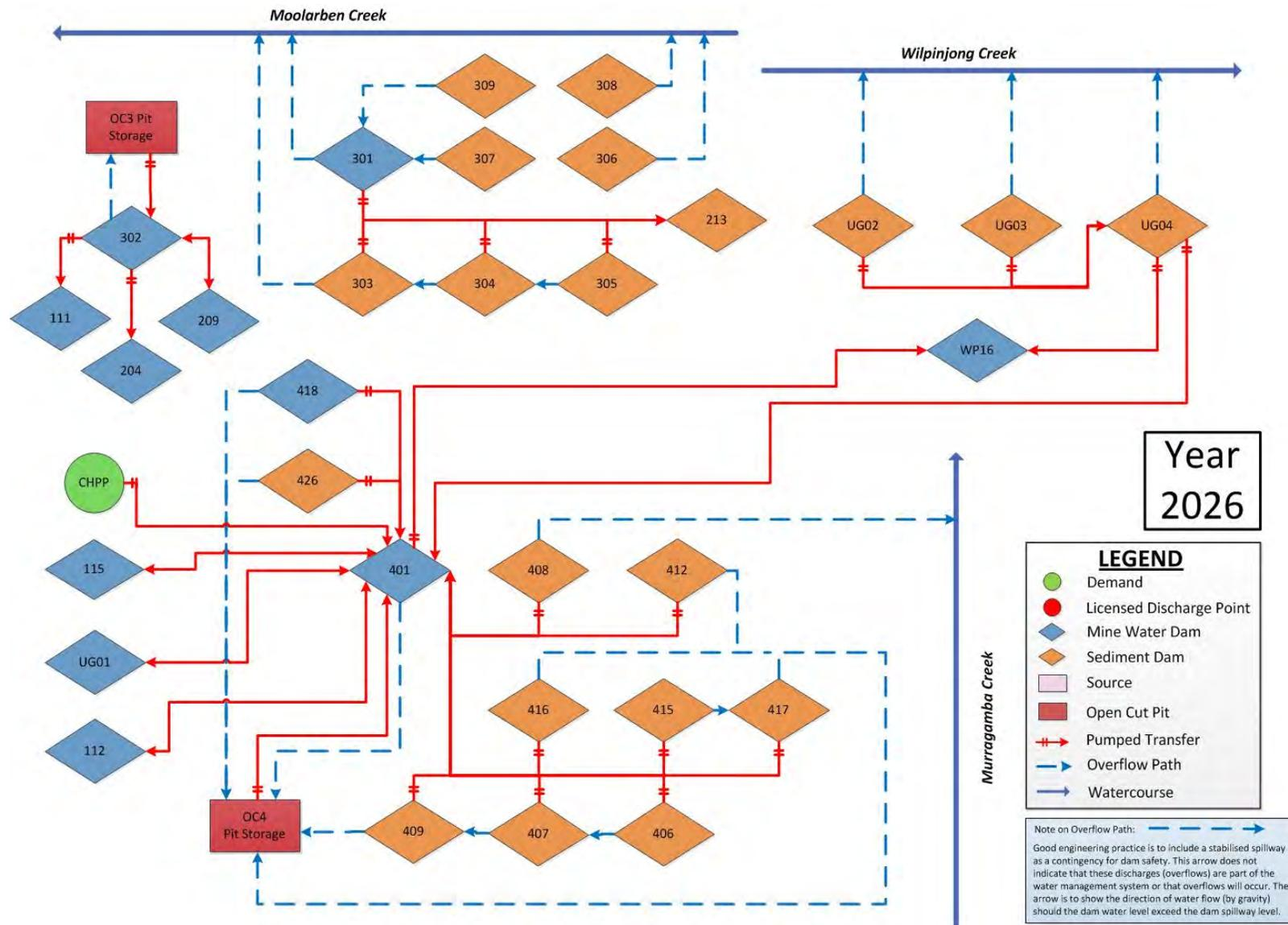
Figure 5.9 - Water management system schematic - OC3 and OC4 (Phase 4)
