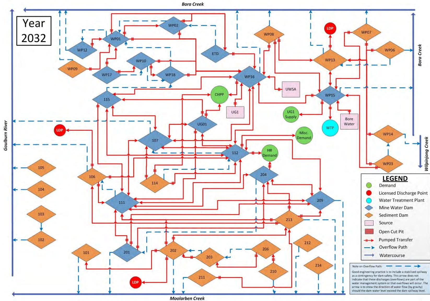
Figure 5.10 - Water management system schematic - WP, OC1 and OC2 (Phase 5)
