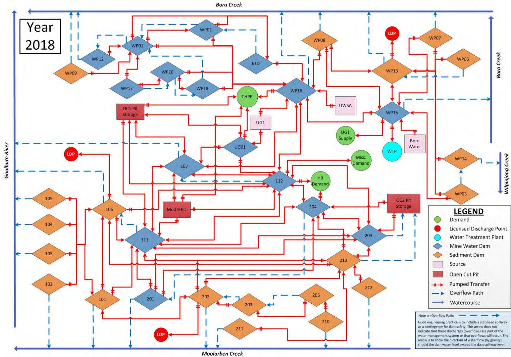
Figure 5.2 - Water management system schematic - WP, OC1 and OC2 (Phase 1)
