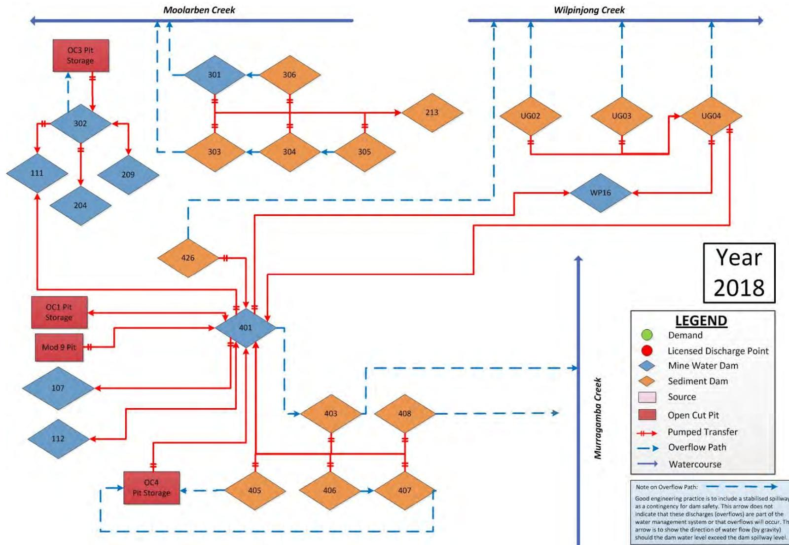
Figure 5.3 - Water management system schematic - OC3 and OC4 (Phase 1)
