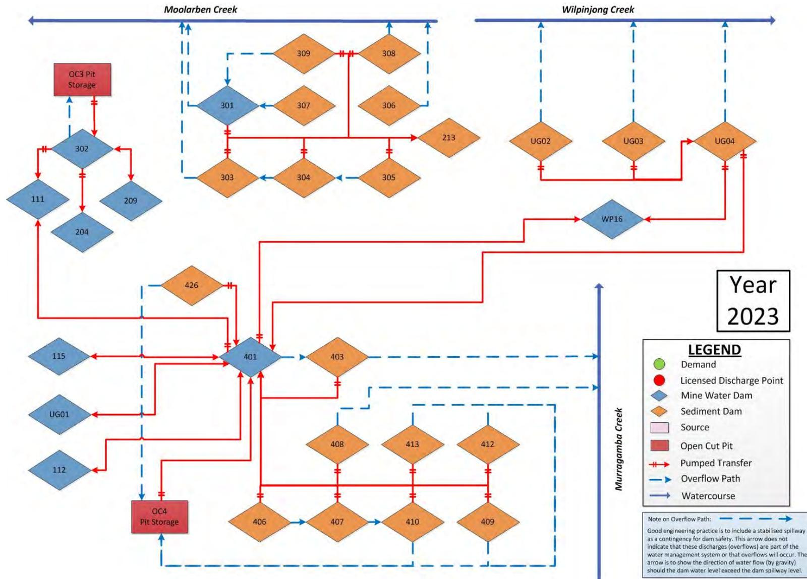
Figure 5.7 - Water management system schematic - OC3 and OC4 (Phase 3)
