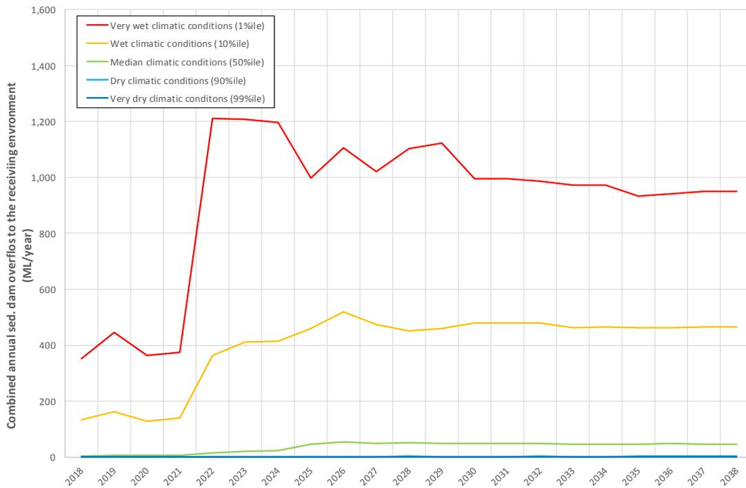
**Figure 6.4 - Forecast annual sediment dam overflows**
