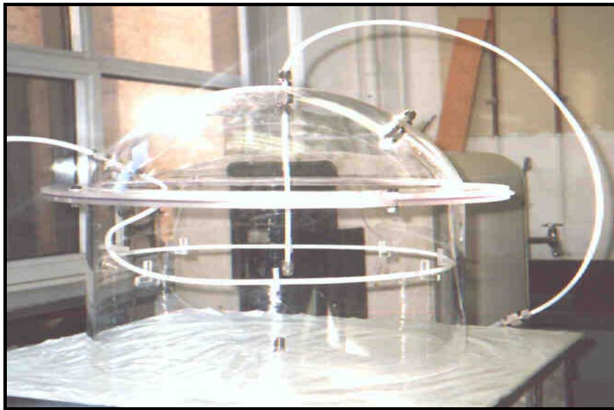
Figure 2-1: A photograph of the isolation flux hood used in the sampling
