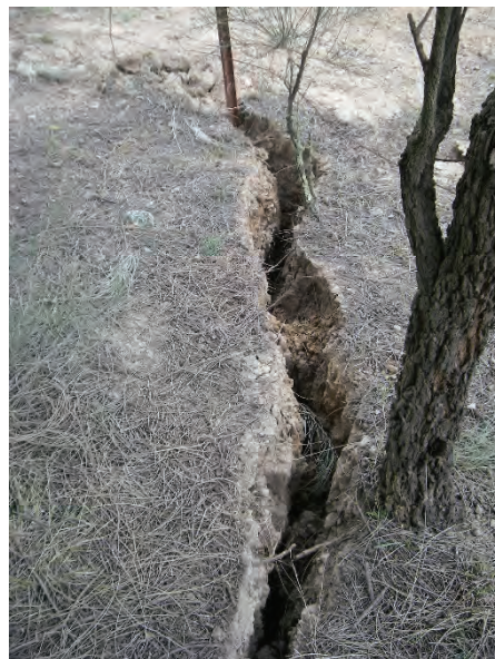
Fig. 5.1 Surface cracking above Blakefield South Mine (multi-seam conditions)
