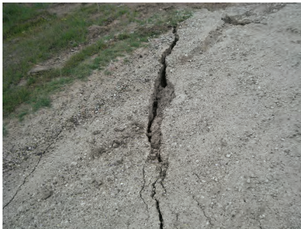
Fig. 5.1 Surface cracking above Blakefield South Mine (multi-seam conditions)
