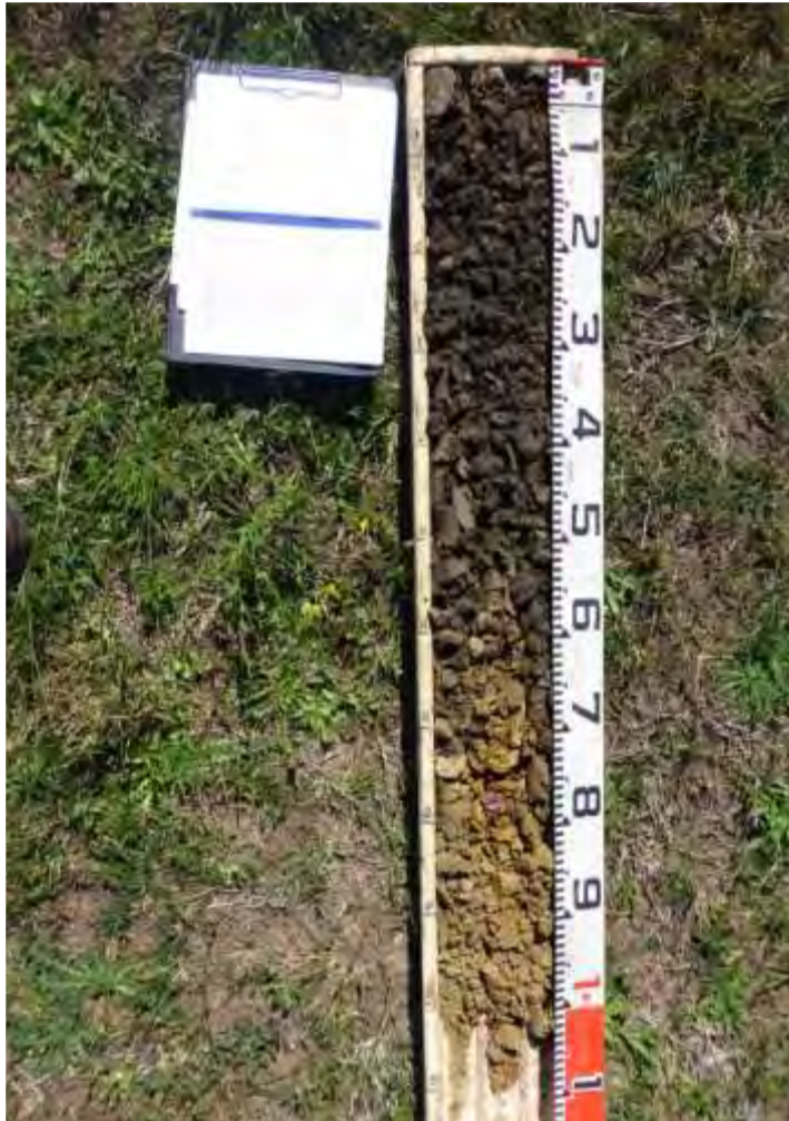
Site 21 - Check Site Self Mulching Black Vertosol
