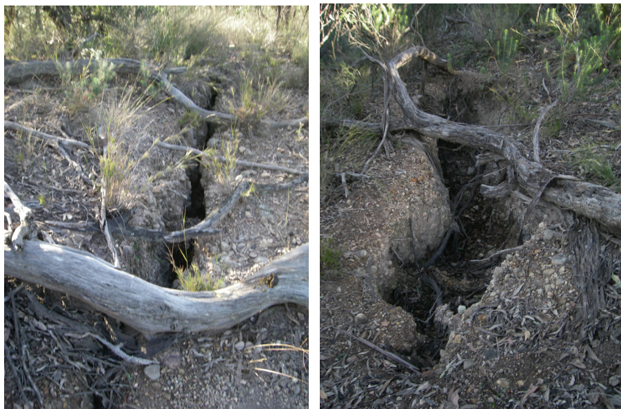
Fig. 5.2 Examples of Surface Cracking on Steep Slopes in the Hunter Coalfield
