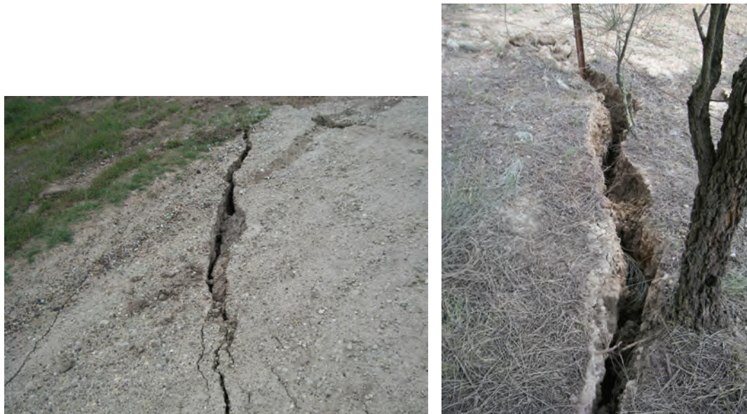
Fig. 5.1 Photographs of Surface Cracking above Blakefield South Mine (Multi-seam)
