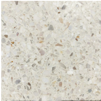
CODE REFERENCE: CON-03 DESCRIPTION: Polished Concrete with Exposed Aggregate MATERIALS AND COLOURS: Colour: White
