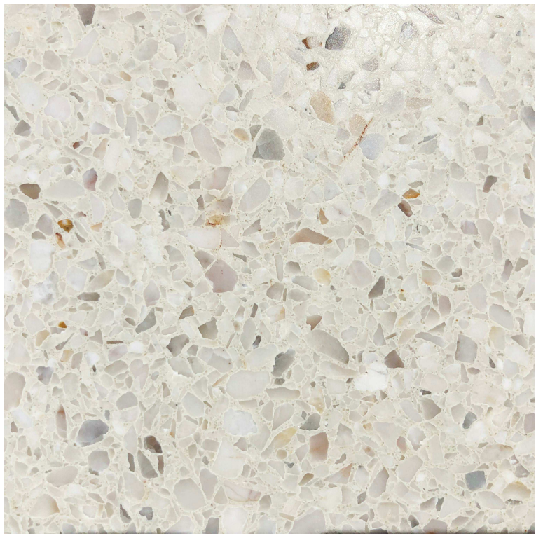
CODE REFERENCE: CON-03 DESCRIPTION: Polished Concrete with Exposed Aggregate
