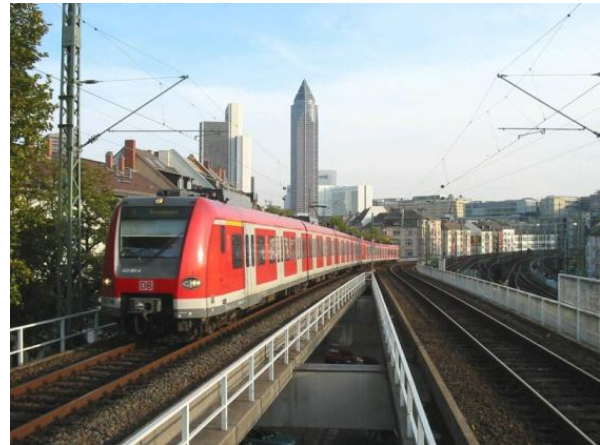
Heavy rail (S Bahn) on elevated clearway to separate long distance trains from urban rail
