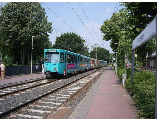
Old style 3 unit tram train (75 m long), used both on low and high platforms and also in tunnels.
