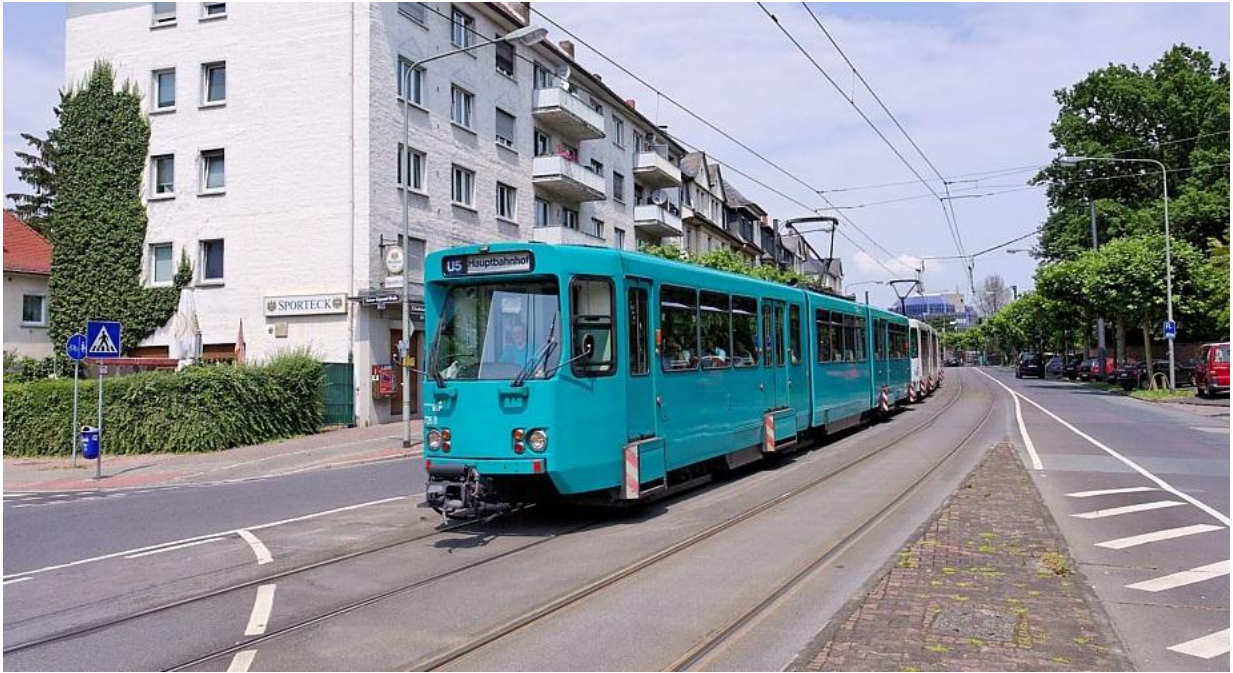
Tram train in Frankfurt using road corridor. Old trams were modified to use high platform tunnels. Many improvisations will be needed once the car culture ends.
