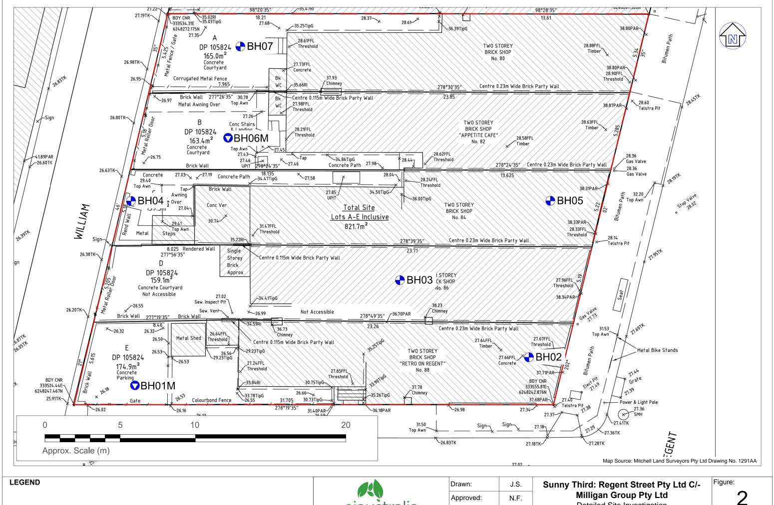
Approximate monitoring well / borehole sample location Approximate borehole sample location Approximate site boundary
