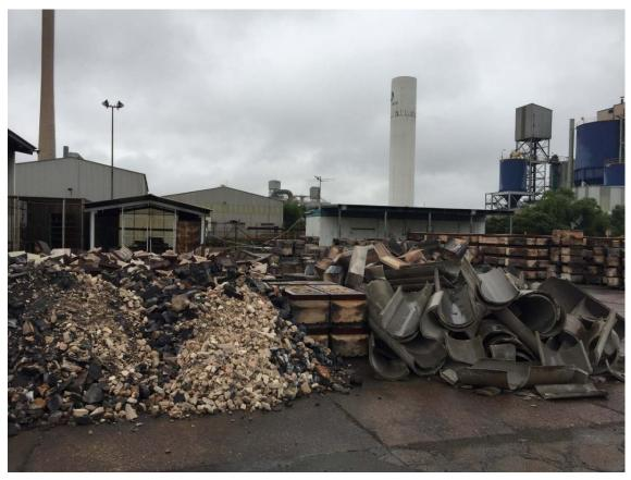
Figure 10 Typical smelter waste stripped, sorted and stored around site
