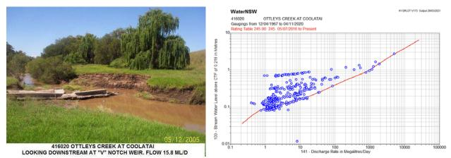
Figure H3 Control weir and comparison of flow gauging and current gauge rating at Coolatai
