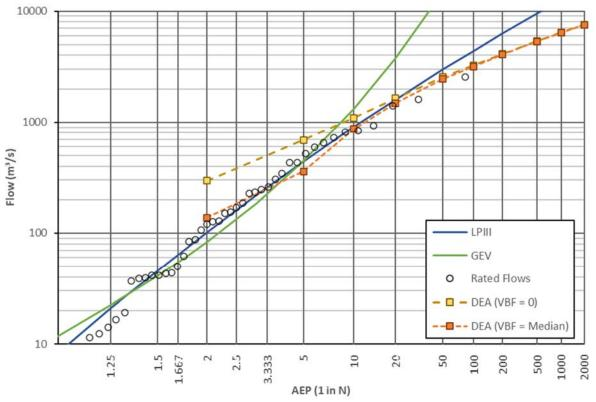
Figure H1 FFA fit and effect of Coolmunda VBF on the DEA flows at Inglewood
