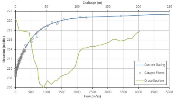
Figure 8.6 Boggabilla stream gauge rating
