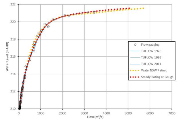
Figure F.5 TUFLOW model results adjusted for dynamic response and proposed steady-state rating
