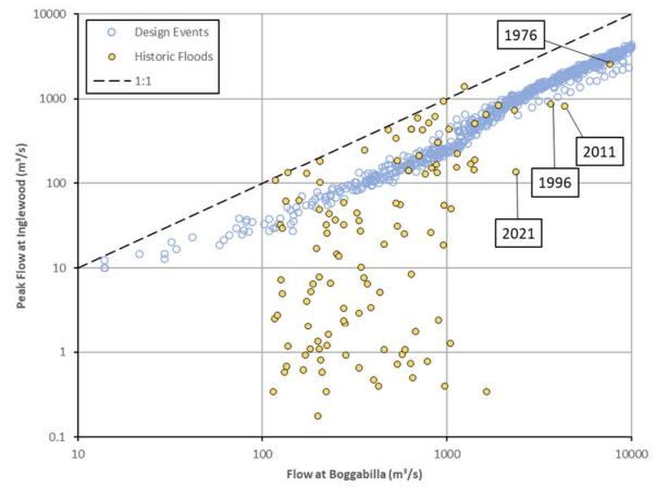
Figure H7 Relationship between total flow upstream of Boggabilla and Macintyre Brook flow at Inglewood
