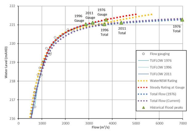
Figure F.6 Proposed Boggabilla rating adjusting for upstream breakout flow
