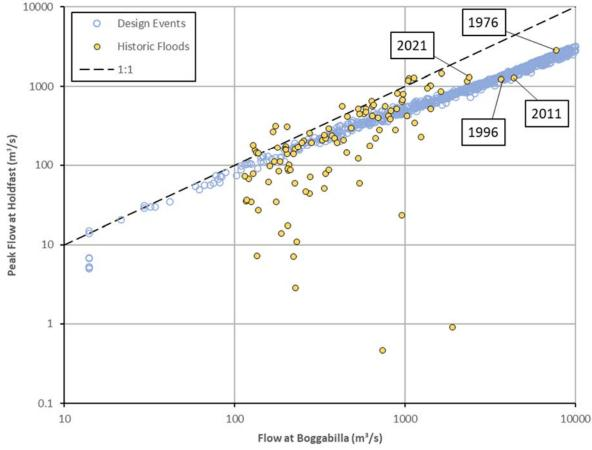
Figure H5 Relationship between total flow upstream of Boggabilla and Macintyre River flow at Holdfast
