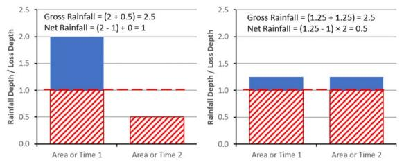
Figure H4 Effect of losses on concentrated vs uniform rainfall
