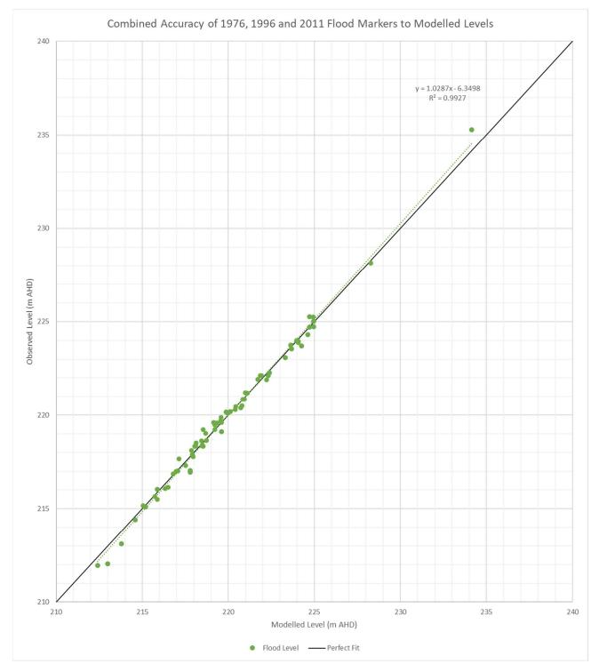
Figure 4-1 General Comparison of Observed and Modelled Flood Levels (FFJV 2021)
