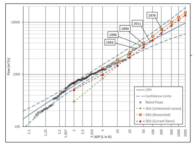
Figure 7-1 FFA & Design Flow Plot at Boggabilla Gauge
