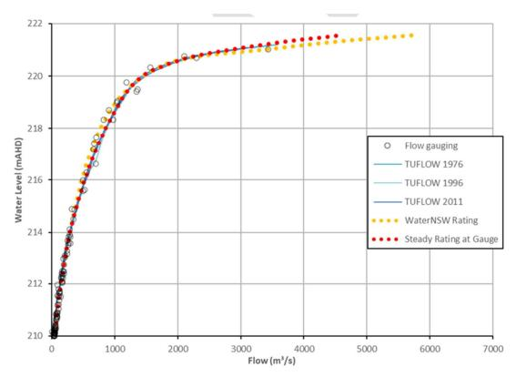
Figure F.5 TUFLOW model results adjusted for dynamic response and proposed steady-state rating
