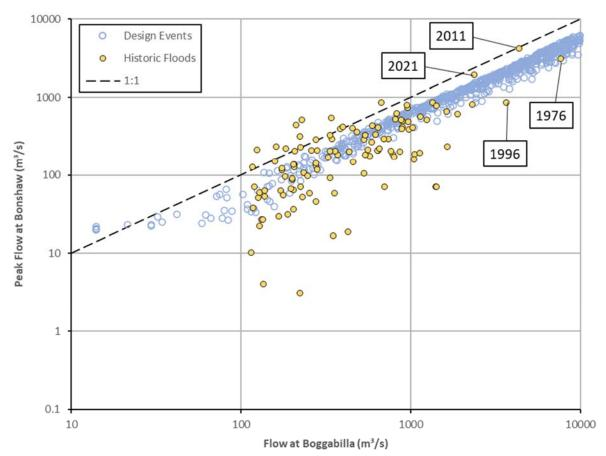
Figure H6 Relationship between total flow upstream of Boggabilla and Dumaresq River flow at Bonshaw
