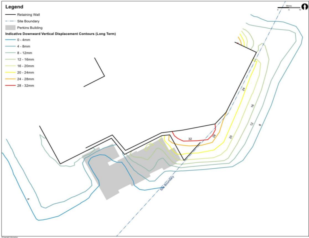
Figure: The predicted vertical settlement at existing ground level.
