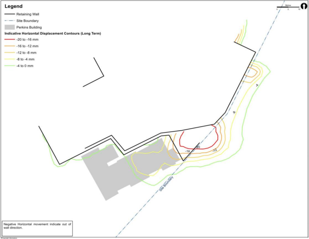
Figure: The predicted horizontal displacement at existing ground level.
