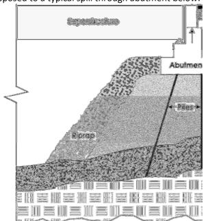
As opposed to a typical spill through abutment below:
