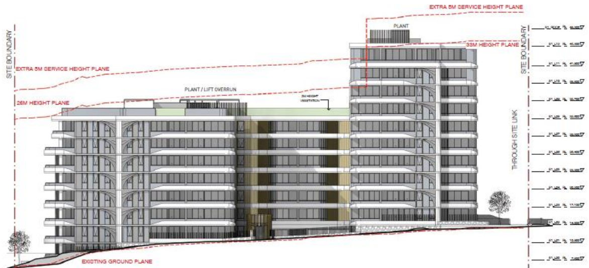
Figure 3 - Height Exceedance No 1 (Northern Elevation)
