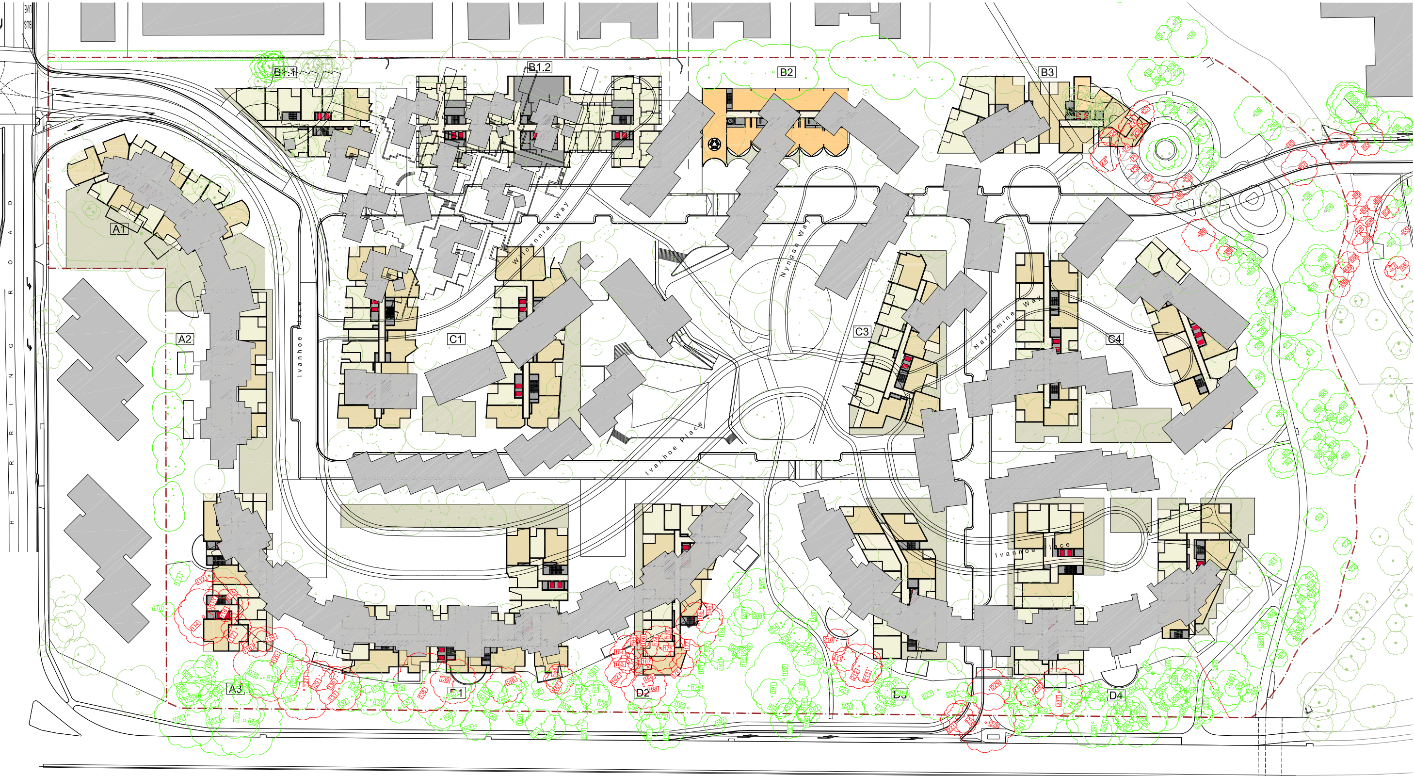
REVISED PROPOSAL COMPARISON TO EXISTING LAYOUT This drawing superimposes the existing buildings and the indicative design scheme to demonstrate that the revised proposal has a similar site coverage but with enhanced open space..
