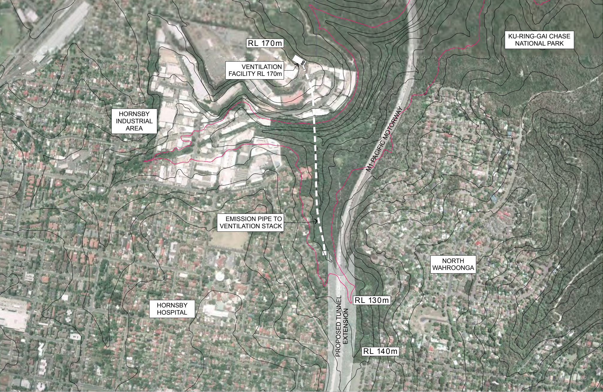
M1-M2 TUNNEL EXTENSION - Proposed emission pipe to ventilation stack in Hornsby Industrial Area approx. RL 170m
