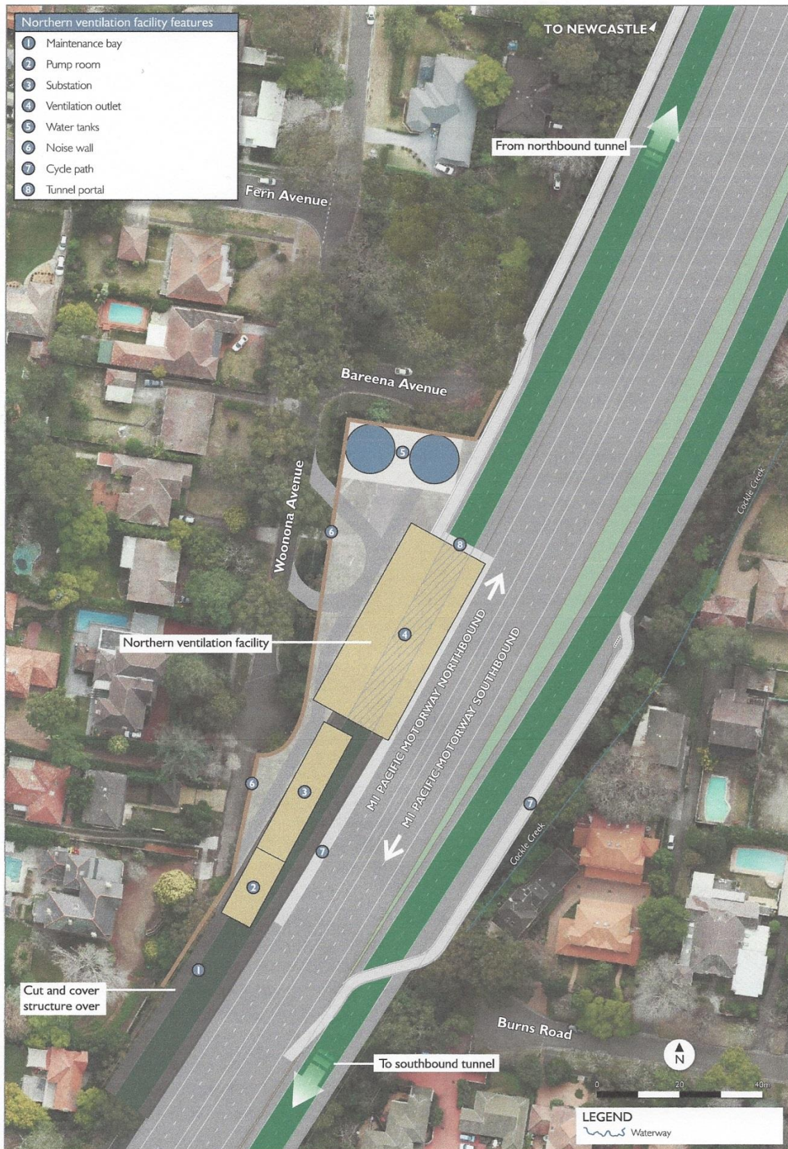
Figure 5-18 Northern ventilation facility operational layout
