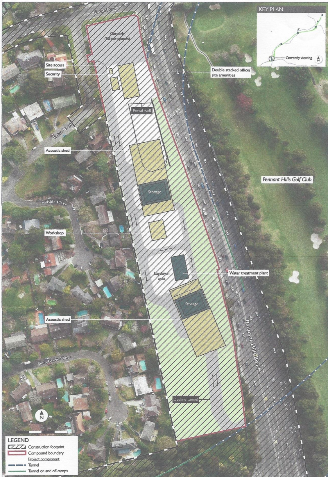
Figure 5-38 Indicative southern interchange construction compound
