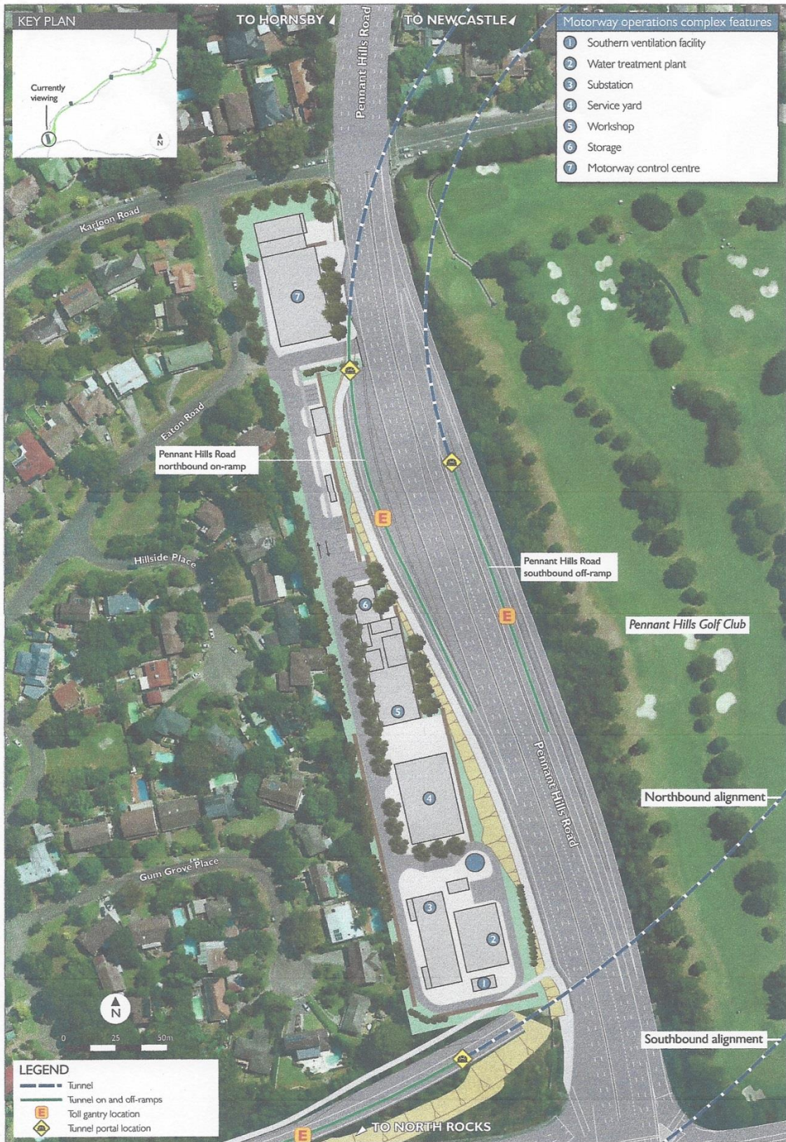
Figure 5-17 Motorway operations complex
