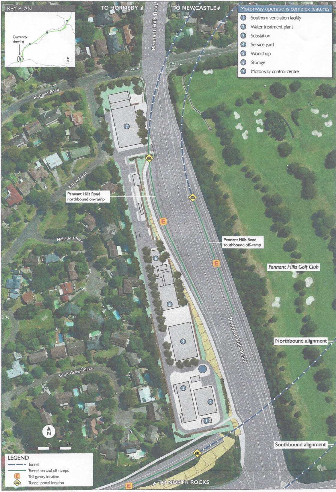
Figure 5-17 Motorway operations complex
