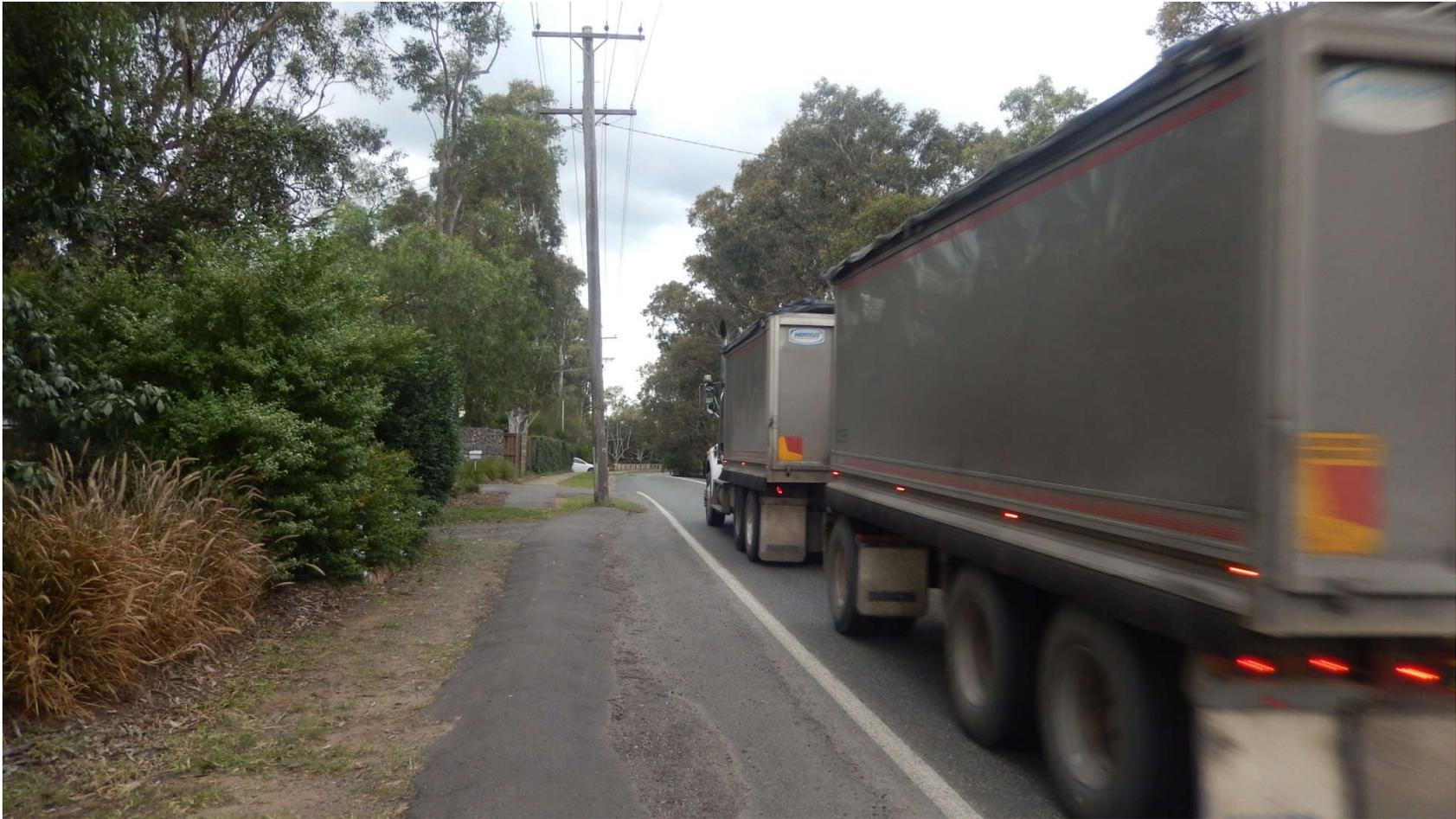
Typical fully laden double quarry truck (50 tons approx) travelling south at 60km/h
