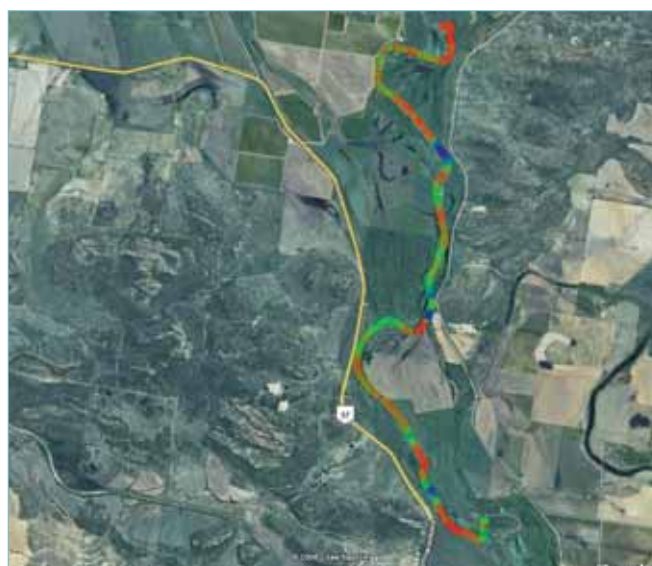
Figure 1. White dotted line indicates the 1 km wide Gap (photo source: Google Earth Professional, 2008). The geo-electric survey depth slice 20 m below the Namoi River, near Gins Leap and the Gap. The blue indicates impervious basement beneath the river; red to green indicates alluvial sediment; redder parts are more saturated and/or more clayey; and the greener parts are less saturated and/or more gravelly. (The unbroken line is the direction of photograph from Gins Leap Boggabri NSW).
