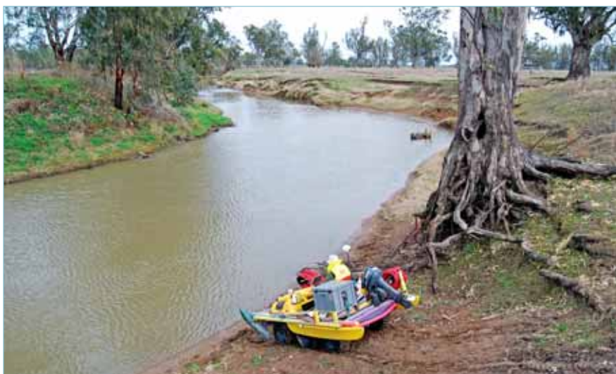
The Argo amphibious vehicle, owned and operated by Groundwater Imaging Pty Ltd, entering the Namoi River north of the Gap. Six driving wheels and a fifteen HP outboard motor allowed the vehicle to progress upstream dragging the 100 m array of electrode senders and receivers. Geo-electric data was recorded continuously and observed on a monitor (photo: K. Crawford, 2008).
