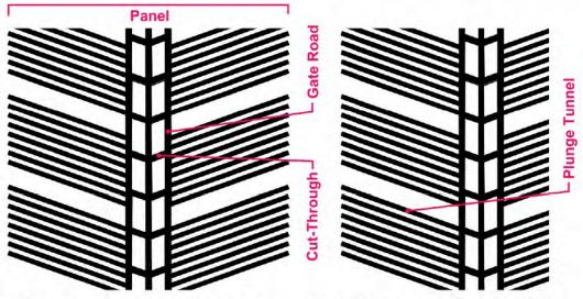
NB: Pillar dimensions and number of plunges differ with cut height and depth of cover. Layout shown is for 130m depth of cover and 3.5m cut height.
