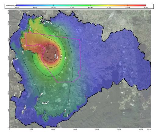
Figure 1.1 – Results from 2013 modelling, extent of drawdown after 5 years for a small 4.5km<sup>2</sup> mine.
