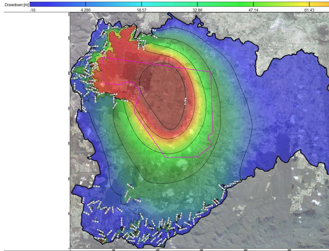
Figure 4.8 – Drawdown in Layer 4, standard values, 20 years elapsed, drain conductance 14.5m<sup>2</sup>/day
