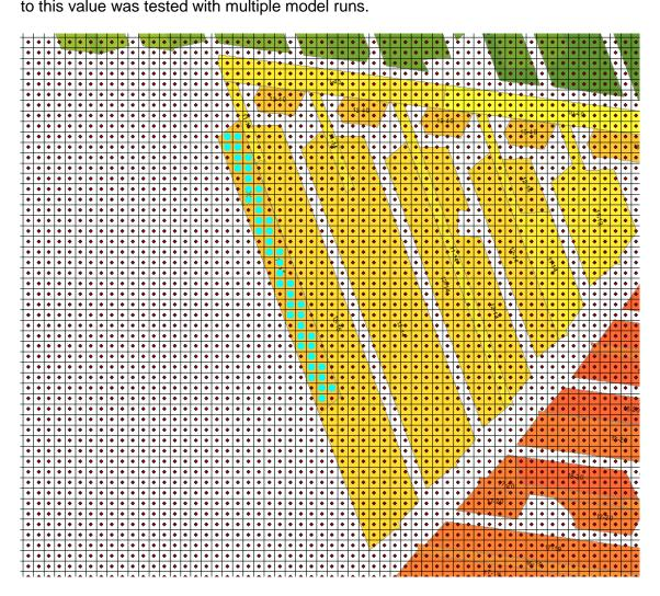
Figure 4.2 – Illustration of the drain cell definition process.
