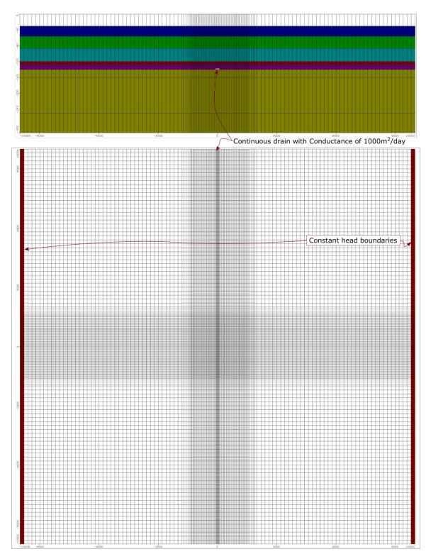
Figure 3.4 – Conceptual 2D model as established in Modflow.
