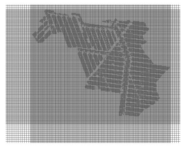
Figure 4.3 – View of mine drain-cells in Modflow
