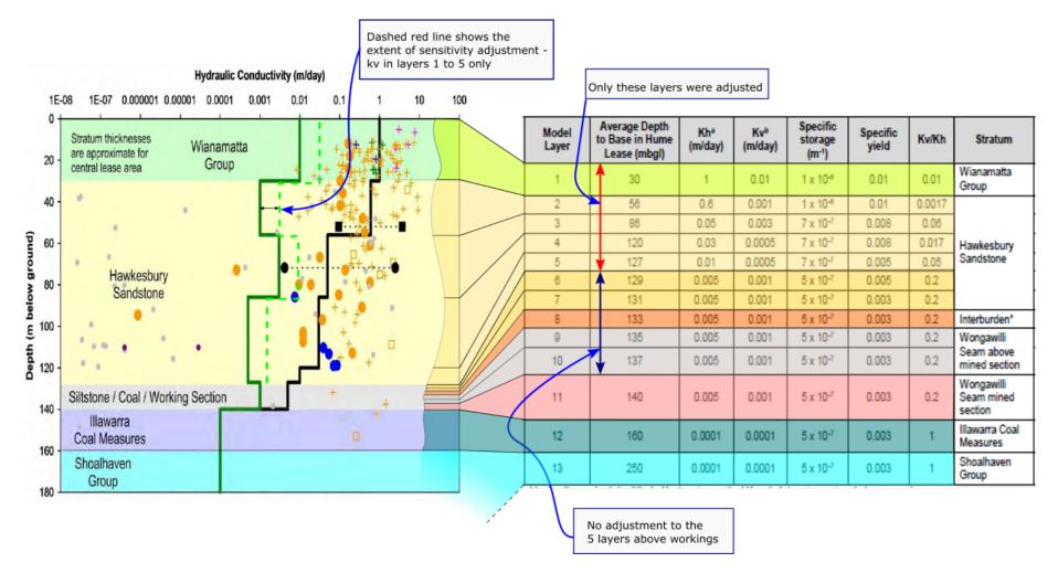
Figure 2.12 – Illustration of the extents of sensitivity to hydraulic conductivity tested in the EIS.
