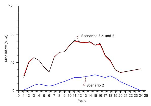
Figure 5.4 – Predicted inflow, Scenarios 2, 3, 4 and 5 showing the effects of mine drain conductance
