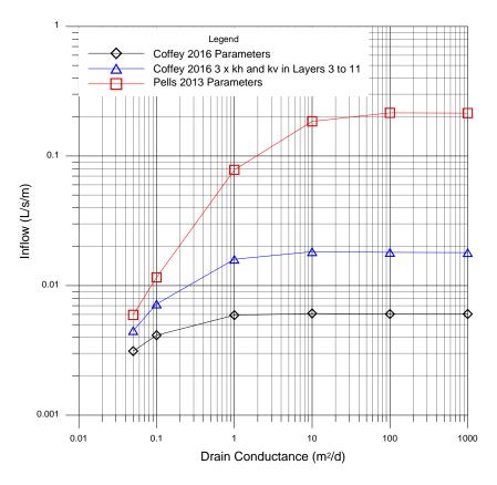
Figure 3.7 – Mine inflows versus drain conductance.
