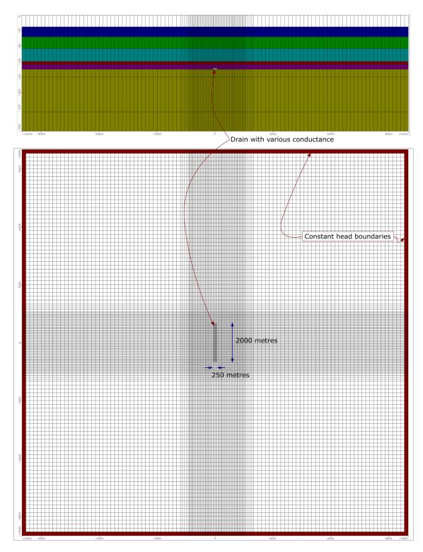
Figure 3.6 – Conceptual 3D model as established in Modflow.
