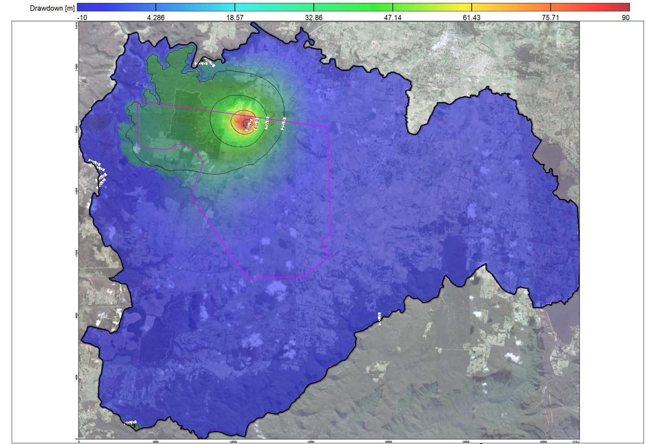
Figure 4.5 – Drawdown in Layer 4, standard values, 1 year elapsed, drain conductance 14.5m<sup>2</sup>/day
