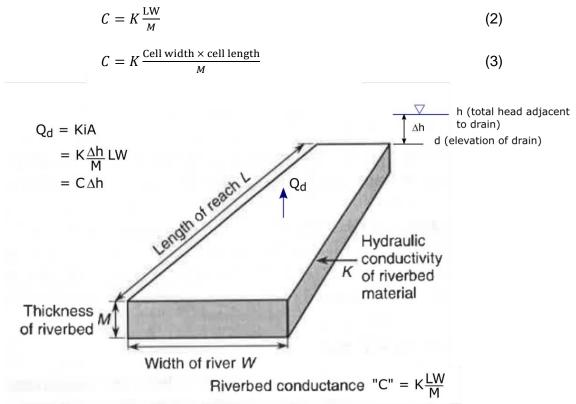
Figure 2.11 – Concept of conductance used in Modflow 'drains' (adapted from Figure 7.17 in Kresig, 2007).
