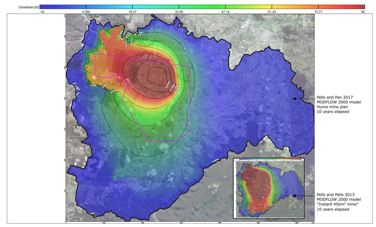
Figure 4.7 – Drawdown in Layer 4, standard values, 10 years elapsed, drain conductance 14.5m<sup>2</sup>/day.
