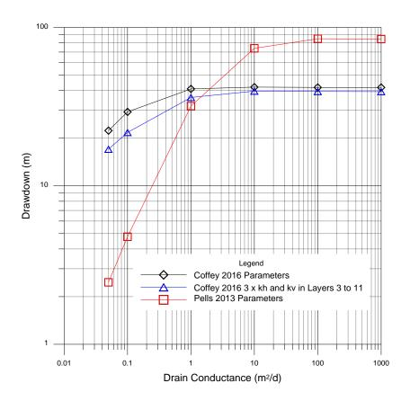
Figure 3.8 – Drawdown above mine, versus conductance.
