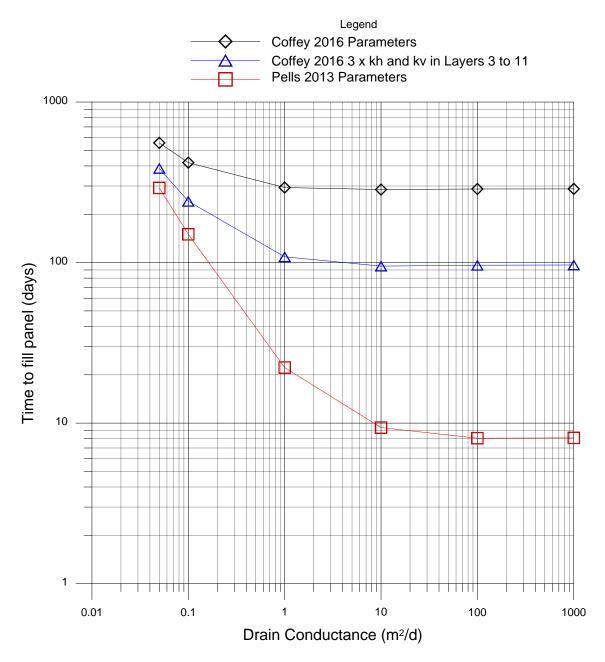
Figure 3.9 – Time to fill a panel versus conductance.
