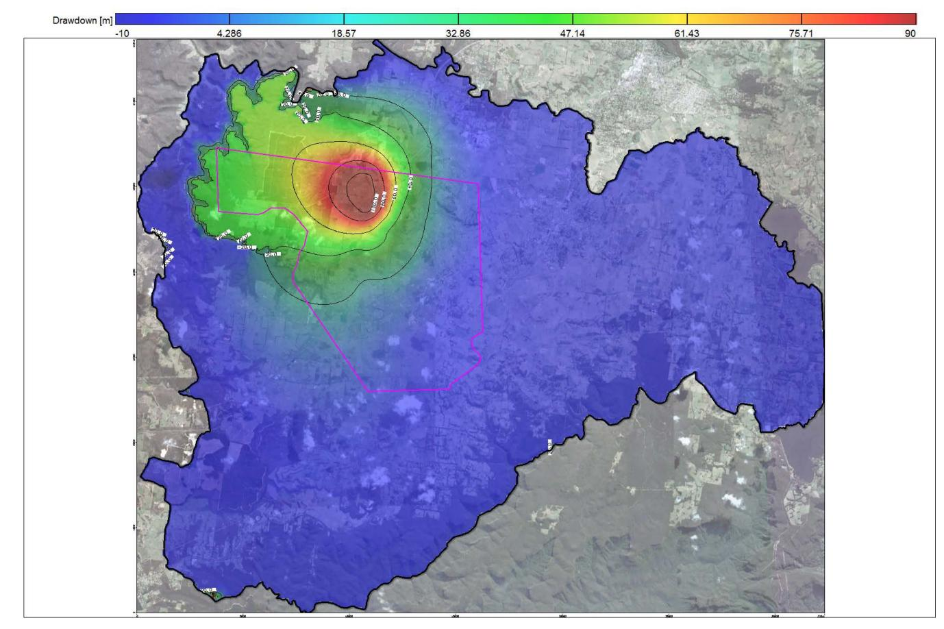
Figure 4.6 – Drawdown in Layer 4, standard values, 2 years elapsed, drain conductance 14.5m<sup>2</sup>/day
