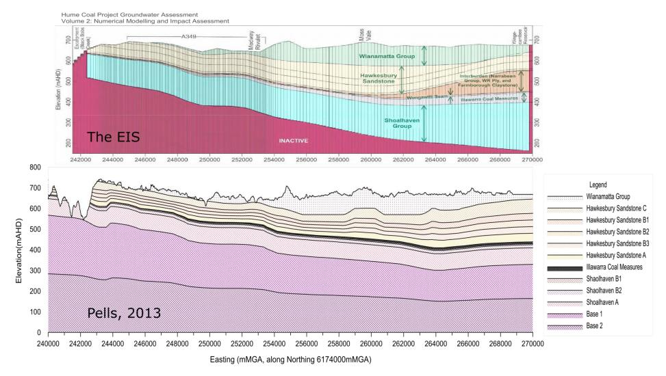
Figure 2.4 – Comparison of cross section from numerical models in the EIS (top) and Pells Consulting 2013 (bottom).
