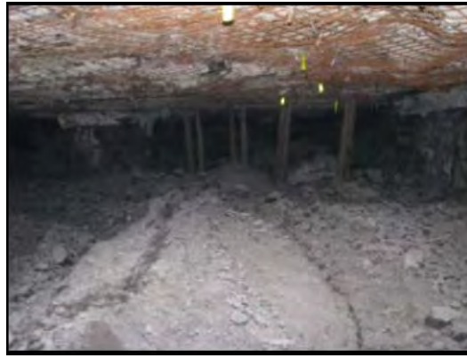
Figure 10. Moderate Floor Heave in 3-North Panel (outbye)
