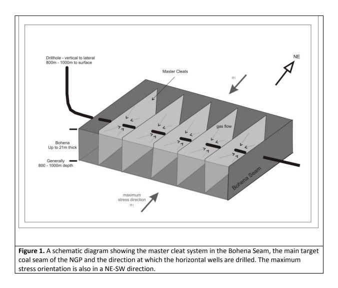
The master cleat system in effect acts as gas gathering structures whereby they provide a pathway, with a very large area, for gas to flow from the coal into the horizontal well and then to the surface. The main orientation of this cleat system, over a large part of the NGP, is also sub-parallel with the maximum stress direction. This has the effect of producing a dilating effect on the cleats thereby having a positive effect on the permeability of the cleats.
