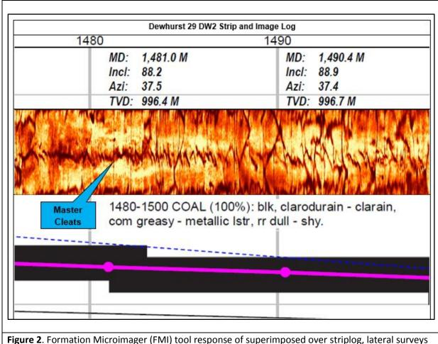
**Figure 2**. Formation Microimager (FMI) tool response of superimposed over striplog, lateral survisions well path and the clear evidence of a master cleat system.
