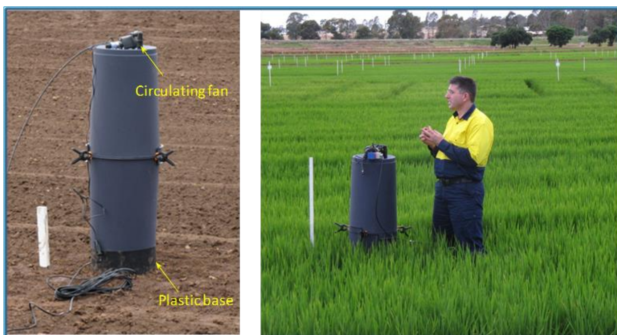
Figure 5.8. Purpose-built flux chamber used for measuring CH 4 emissions from rice
