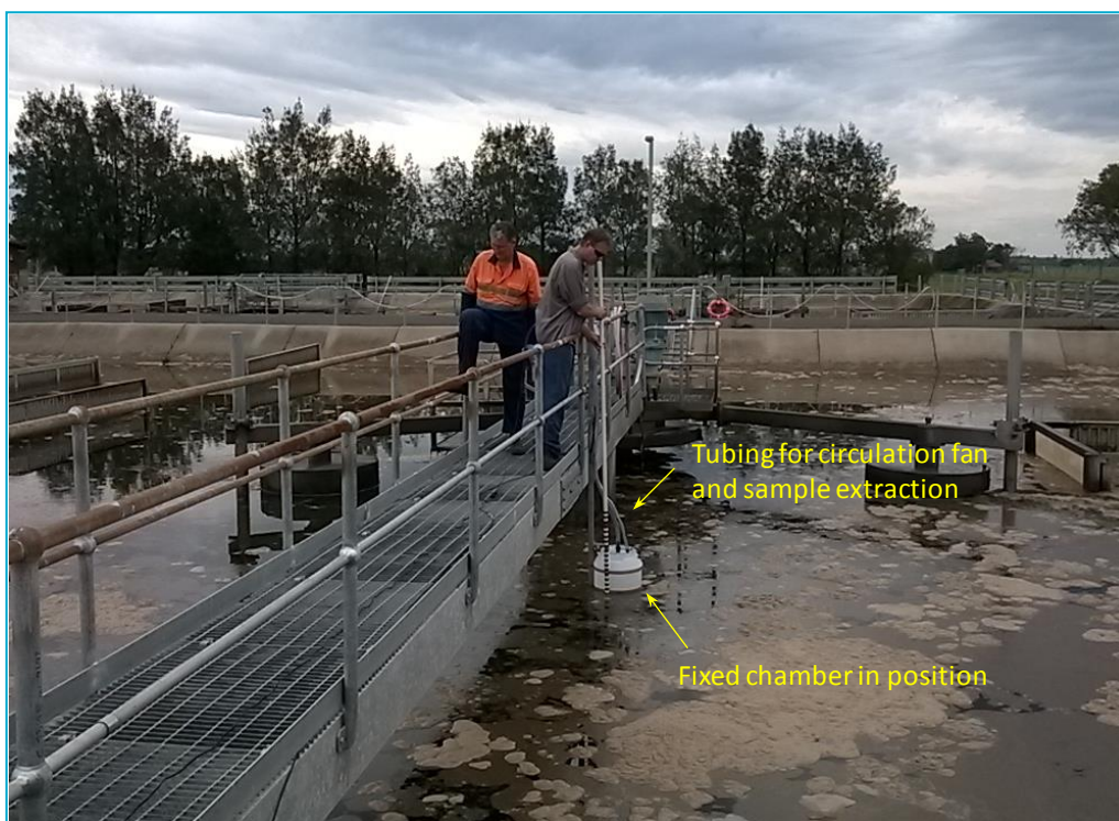
Figure 5.6. Fixed flux chamber in operation at the Singleton wastewater treatment plant
