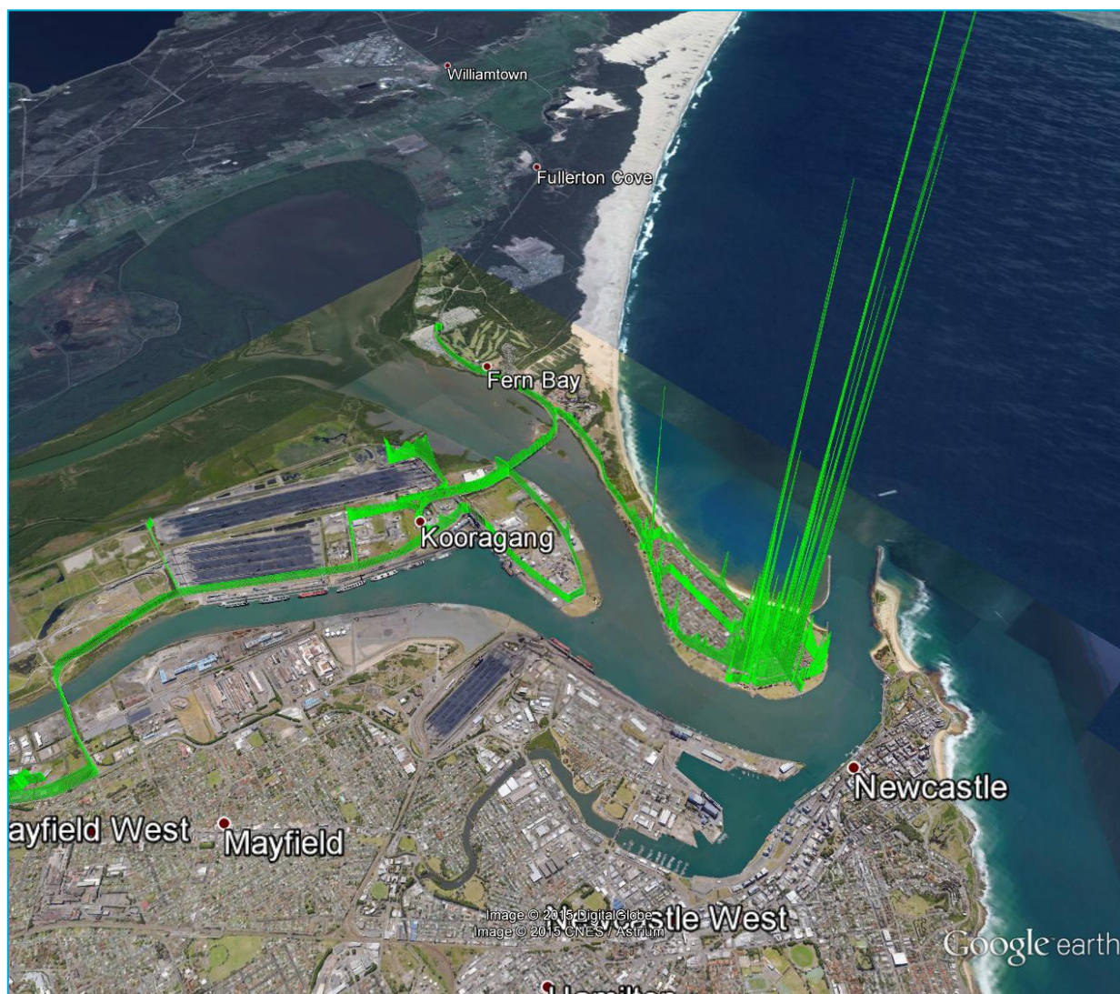
Figure 6.4. Mobile survey of \text{CH}_4 concentration in the Newcastle region near Stockton. The maximum \text{CH}_4 3-s average peak measured in Stockton was approximately 22.0 ppm.
