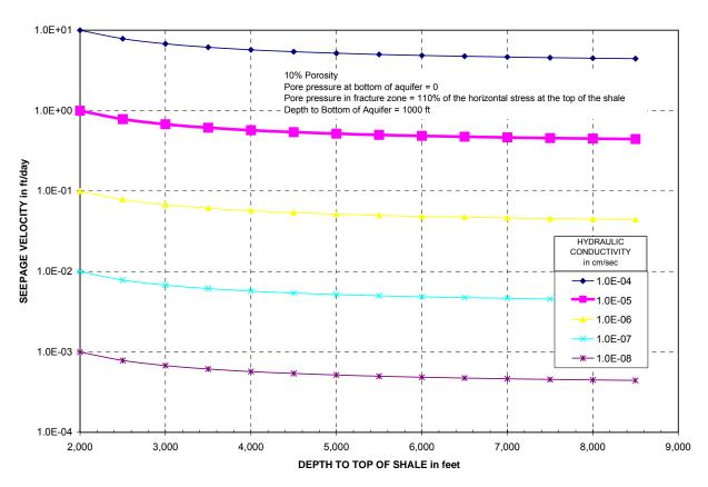
Figure 2: Seepage velocity as a function of hydraulic conductivity
