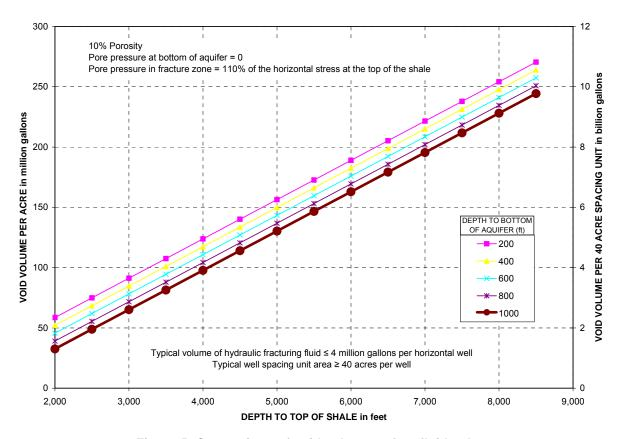
Figure 5: Comparison of void volume to frac fluid volume
