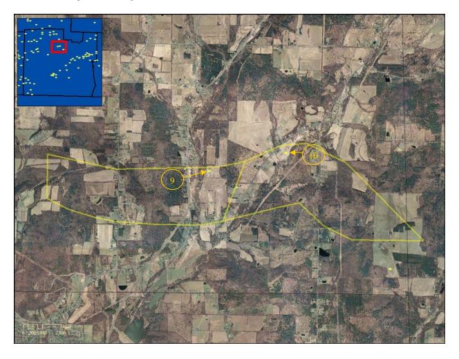
Photos 6.16 Well #9 (Hole number 23228) was drilled as a horizontal Trenton-Black River well and completed in 2006. The well was drilled to a true vertical depth of 9,461 and a true measured depth of 12,550 feet. The well unit is approximately 622 acres.
