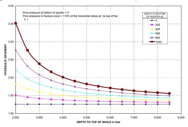
Figure 1: Average hydraulic gradient during fracturing
