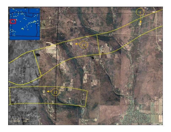
Photos 6.19 Well #11 (Hole number 22831) was completed in 2000 as a directional well to a total vertical depth of 9,824 feet. The drill site disturbed area was approximately 3.6 acres which has been reclaimed to a fenced area of 0.5 acres.
