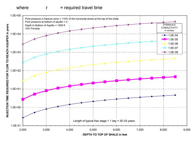
Figure 3: Injection time required for fracture fluid to reach aquifer as a function of hydraulic conductivity
