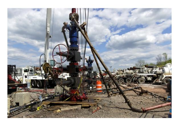
Photo 5.24- Three Fortuna Energy wells being prepared for hydraulic fracturing, with 10,000 psi well head and goat head attached to lines. Troy PA. Source: New York State Department of Environmental Conservation 2009
