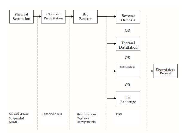
Figure 5.7 - One configuration of potential on-site treatment technologies.
