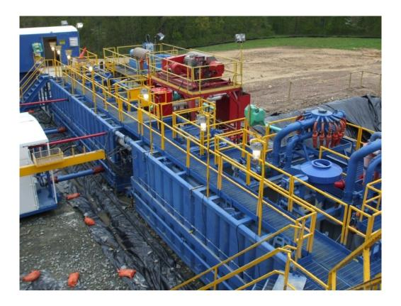
Photo 5.16 - Drilling rig mud system (blue tanks)
