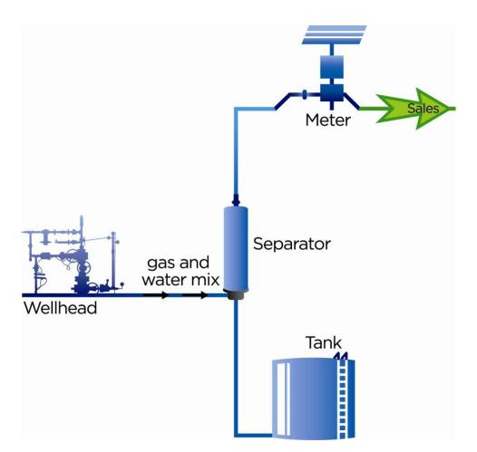
Figure 5.8 – Simplified Illustration of Gas Production Process
