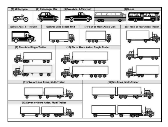
Figure 2.16 - FHWA Vehicle Classifications (New August 2011)
