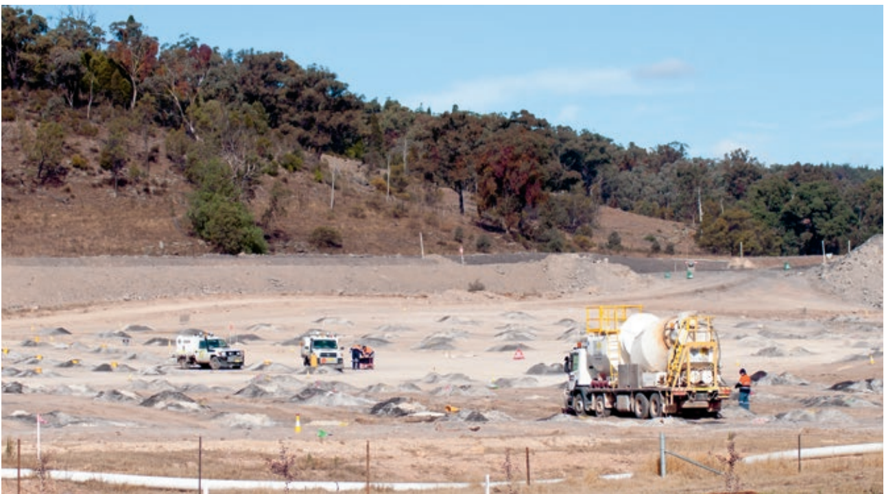
Laying explosives at Moolarben. Photo: Max Phillips
