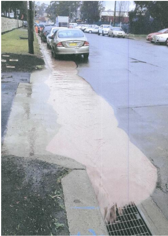
PLATE 9: Sediment laden runoff from Enviro Recycling running down Violet Street and into stormwater drains.
